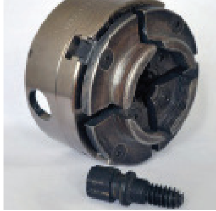
Scroll chuck with woodworm screw
