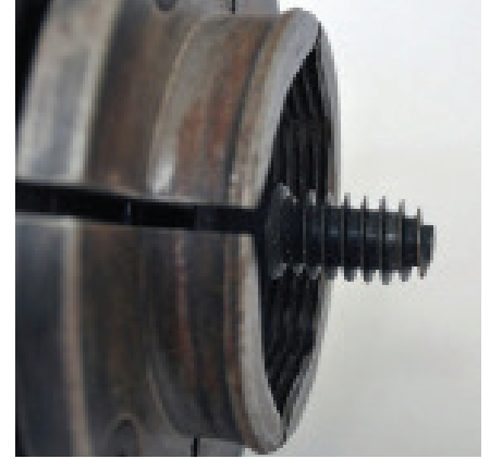
Scroll chuck with woodworm screw
