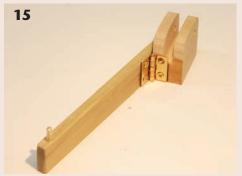
Install the hinges on the body, aligning the hinge flaps with the center line. You may need to improvise a bit to brace the components until the CA begins to cure. Seat the hinge screws.
