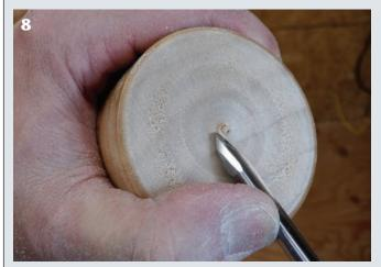
Use a parting tool to remove the holder from the lathe. Clean-up the nub with a sharp gouge or knife.
