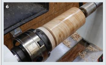
Sand to completion and apply a finish to the exterior.
