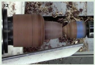
Remove the cap and shape as much of the exterior of the acorn as you can reach. You will need to reverse chuck it (see sidebar) to finish shaping and sanding the tip.
