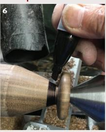
Using the tailstock for support, shape Add a hat band using a permanent marker. Don't use a worn pen, which may leave a ragged line.
