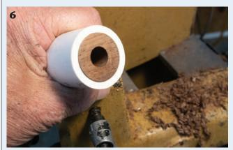
Turn a short wood plug to fit the bottom end of the handle. The drawbar passes through this plug, so drill a hole through the center before securing the plug in the bottom of the handle with adhesive.
