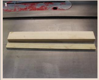
Start with hardwood stock and a ripping cut at the table saw.
