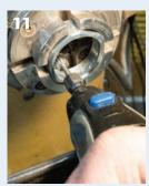
A 1" compression fitting can be modified to work as a ferrule. This requires a very slight reduction of the OD of the pipe as well as enlarging the interior of the nut with a grinder.
