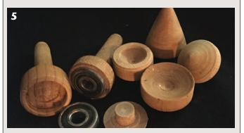
Shopmade tailstock live centers, made possible by the use of ball bearings, expand the range of work-holding options at the tailstock end of the operation. These are based around a turned Morse taper tenon inserted into the tailstock quill.
