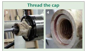
Tap internal threads using a commercially available tap and pressure from your tailstock.
