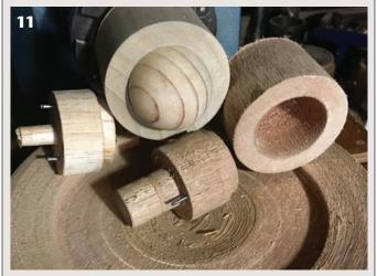
Taking advantage of close tolerances, friction jigs and drives can hold spheres and drive spindles or vessels. If an object needs to be re-chucked multiple times during a project, a friction drive can be a time saver.
