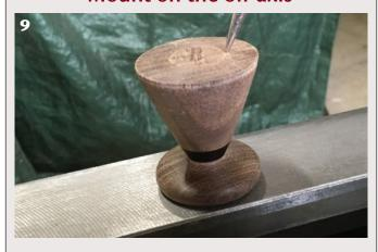
Mark the location for remounting your blank off-axis. Moving a section of the blank away from the axis of rotation means it is more likely to be removed during turning.
