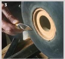
Charge a leather-faced disk with honing compound to make a quick and efficient stropping disk.
