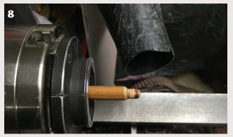
Use a dowel to make a shopmade friction drive for your hat. Taper the end to fit securely in the hole in the base of the hat blank.
