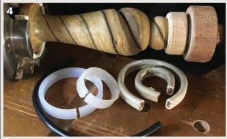
Position chuck jaw inserts made from a cutting board or scrap insulated wiring between the jaws and work piece to prevent the jaws from marring the work.
