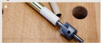
While many mandrels can accommodate a variety of pen kits, pen mills (or barrel trimmers) are specific to certain tube sizes. Lacking the correct pen mill (or barrel trimmer), the author transferred dimensions from the pen tubes to the blanks using a caliper. While not as convenient, the results are just as precise.
