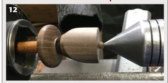
Refine the top of the hat with a series of shearing cuts, made either with the long tip of a skew chisel or a spindle gouge presented on its side.
