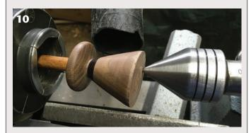
Angle the blank on the friction drive and secure it in place using the tailstock in the off-axis location. Snug the tailstock, but don't overtighten it and split the blank or break the friction drive.
