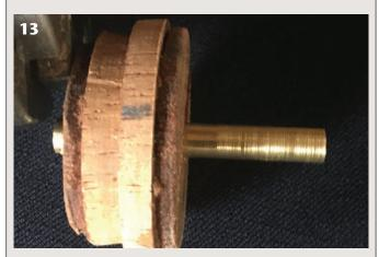
Metal insert tubes (for pens, for example) need to be scuffed to give adhesives a bonding surface. This leather pen tube holder makes the task easy and keeps your fingers out of the way of the abrasives.
