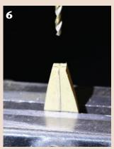
Shape the pivot using abrasives (the author used a disk sander). With the pivot held securely in a vice or clamp, drill a hole to match your metal rod about 5/8" deep in the narrow end.
