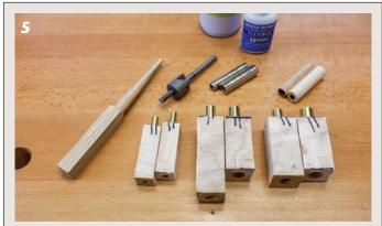
Some degree of organization is critical when turning pens. Blanks for the three kits are grouped by kit (they aren't interchangeable), with each set marked to help keep track of grain alignment.
