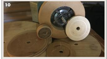
Adding surface area around chuck jaws allows the chuck to function as a faceplate. The system includes a support ring and backing plates, all easily made from sheet goods.
