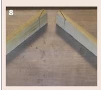
Lay out the bevels and drilling locations and cut (or shape) the bevels. Drill 3/64" holes, 3/8" deep near the tips to receive the brass brads.
