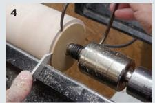
With the blank mounted in your four-jaw chuck, transfer your external measurement using your caliper and a parting tool to several locations along the length of the blank.
