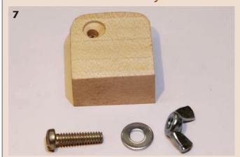
Trim the body to shape and drill a 3/16"-diameter hole through the side. Countersink the left side for the head of the machine screw pivot.
