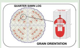
You'll want to turn these forms in facegrain orientation, which may seem odd as their length and chucking method would make you think "spindle." However, the suggested orientation creates the strongest threads.
