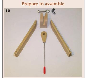
Lay out all of the components to prepare for assembly, including the two legs, the pivot with its rod, and the body that connects the legs and pivot.
