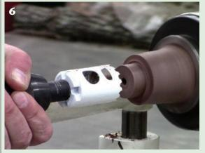
After bringing the bottom to round, use a hole saw to create a spigot on the end. Shape a perpendicular shoulder at the base of the spigot.
