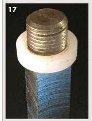
With a little help from a metal shop, thread the end of a metal billet to match the internal threads of your chuck adapter. You can now move your chucked form to a vice for carving, pyrography, painting, or other forms of embellishment.
