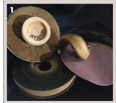
Flexible-grid sanding disks and leather-faced strop (lower left). The author sanded the intricately curved form in the center using this system.
