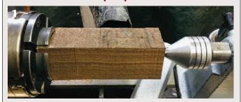
Mount your blank in the chuck jaws and bring up the tailstock for support.
