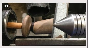
Shape the sweep of the hat, taking light cuts from the perimeter of the "ghost" edge as the off-axis blank rotates through space.
