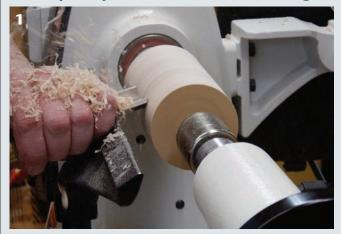
Mount your blank between centers and bring it to round with a spindle roughing gouge.
