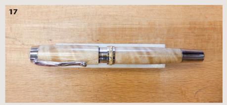
Tolerances are tight and you want to avoid having to pull pieces apart because you put them in the wrong place; lay out and double check the sequence of components before assembly.
