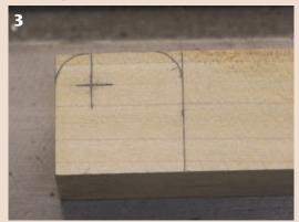
With a standard blade back on the saw, crosscut a 1-1/4" length for the body of the base.
