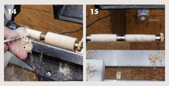
Use a spindle roughing gouge to knock the corners off the blanks and quickly brings them to round before switching to a skew chisel for refined cuts. Despite the diminutive size of the turning, artistic expression is still possible; note the understated but elegant curves.
