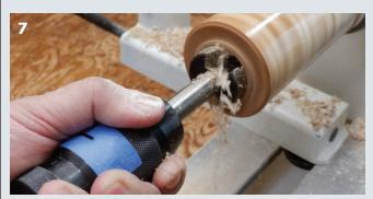
Using your Forstner-style bit (or bits), bore out the interior of the holder. Be sure to leave enough material in the bottom for parting.
