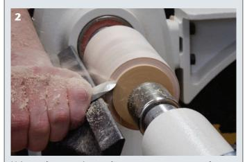
Using a skew, parting tool, or a square scraper, make a peeling cut to create a tenon to fit your four-jaw chuck.
