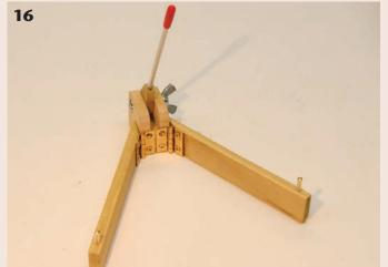
Use the #10 machine screw with matching washer and wing nut to attach the pivot.
