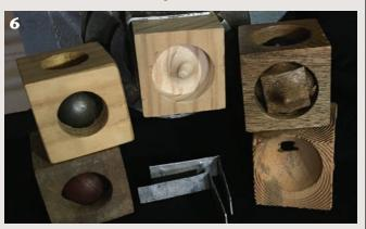
Chuck jaws will hold square stock, but not without marring the surface. Jaw inserts to secure a small cube for turning are easily made by bending narrow aluminum stock.
