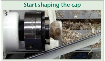
Use a spindle gouge to shape as much of the exterior of the cap as you can easily reach.
