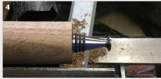
Turn the stopper in by hand, forcing the stud to cut its own threads as you proceed. The stopper should seat against the bottom of the blank without a visible gap.
