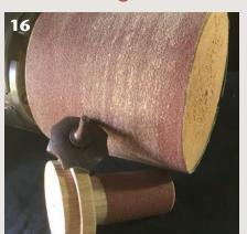
Chuck-mounted sanding drums are handy in the woodshop and can be used on anything from curved table legs to adding decorative elements to a turned form. Add foam backing material if you need a less-rigid surface.
