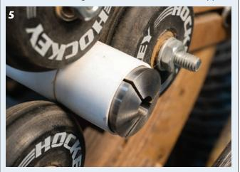
Test fit the collet. The taper doesn't have to be perfect, but you do need to be able to seat the collet.
