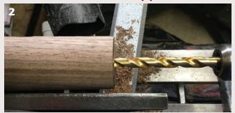
Drill the bottom of the hat blank to receive the threaded stud on top of the stopper.
