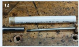
Lashing the end of the pipe with string set with a soaking of CA glue is a low-tech approach to a ferrule.
