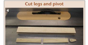
Cut two 4-1/2"- (11cm-) long pieces from the 1/4" strip for the legs and a 1-1/4"- long piece for the pivot using mitre saw or handsaw.
