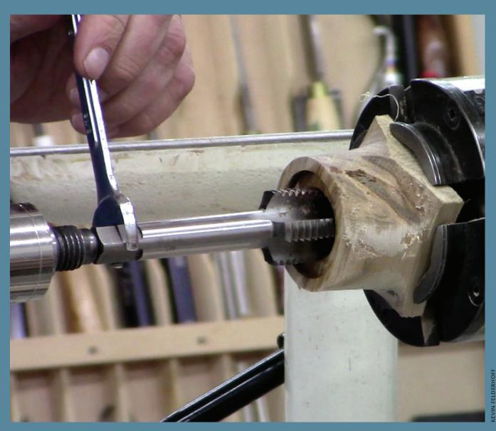
Taps to create threads in wood are available in numerous sizes and can greatly expand your bag of woodworking tricks. Taps that correspond to the size and pitch of your lathe's drive spindle will allow you to make jigs that will thread right onto your lathe (see Ernie Newman's article, starting on **page 34**). You can use the same tap to thread a small box lid (see Kevin Felderhoff's article, starting on **page 20**).
