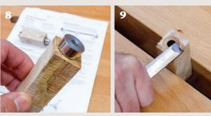
A larger-than-normal bushing on the Panache pen sent the author looking for a solution to trim the blank end perfectly perpendicular to the axis of the barrel (usually accomplished with a barrel trimmer). The solution was a razor-sharp chisel, a vise, and a steady hand.
