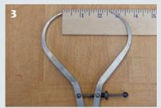
Set a caliper to your final dimension. If you're not confident about your turning skills, add a fraction of an inch to your diameter to give yourself room for correcting tearout or tooling problems.
