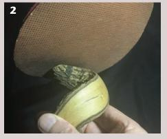
Extending the backing and abrasive sheet beyond the perimeter of the wood backing surface allows the sanding surface to flex and conform to convex shapes.
