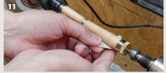
A skew chisel almost always leaves a better surface than a spindle gouge, needing only a quick run through the abrasives stack to bring the pen to finish-ready.
