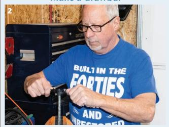
If you have the appropriate tap and die, you can easily cut threads on the end of a rod to create a drawbar. Alternatively, buy a piece of all thread rod long enough to suit your handle.
