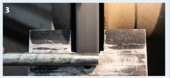
If you cut your own threads, you will need to reduce about 3/4" of one tip's diameter of a standard 7/16" rod to about 0.43" using a bench grinder.
