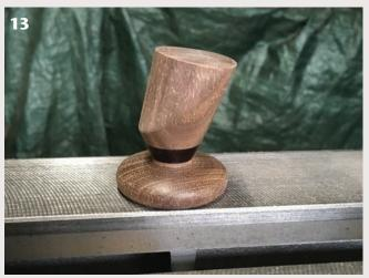
Remove the nub from the top of the hat with a chisel or carving knife, sanding the area to blend the surfaces.
