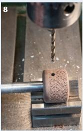
Drill a hole through the tightening nut and into the drawbar and pin the two elements together to help secure this connection.
