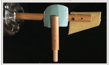
Attempting to sand the interior of small hollow forms and boxes by hand at the lathe is inviting injury. The fly sander holds small strips of abrasive, extends your reach, and keeps your fingers well out of harm's way.
