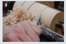
Use a skew and paring cuts (if necessary), finishing with light passes and shearing cuts to reduce your cylinder to the marked dimensions.
