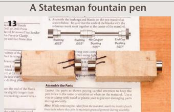
Verify bushing orientation before starting, especially in a kit of this style with three subtly different bushing sizes.
