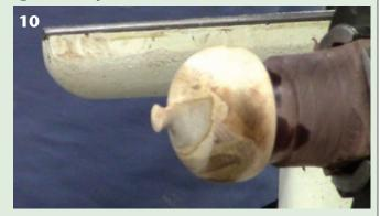
Thread the cap onto the bottom and finish shaping it. Use the tailstock for support up until the last cuts on the tip. A shopmade cap on the live center prevents marring the top of the acorn.
