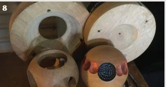
Sphere-holding jigs essentially clamp the ball between two pieces of wood with an opening for turning access.
