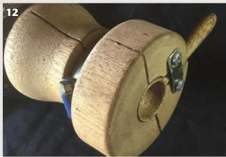
Spoons and some scoops need to be mounted on two axes for turning—one for the handle in spindle orientation, one for hollowing the facegrain bowl. This handy jig holds the form for hollowing the bowl with a slot to accommodate the handle.
