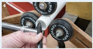
Form a taper on the inside of your PVC handle using a spindle or bowl gouge and a scraping cut. A steady rest is essential for working this far out from the chuck's support.
