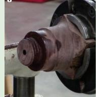
Cut a slight chamfer on the end of the spigot and use a die to cut threads on the spigot. You'll also need to undercut the last thread with a narrow parting tool.
