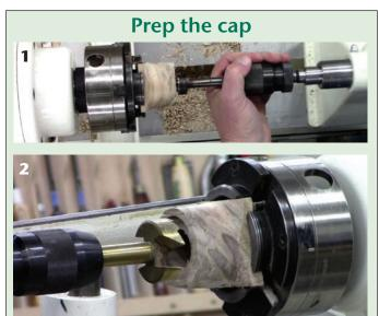
Bring the cap blank to round and use a drill chuck to drill stepped holes in the bottom.
