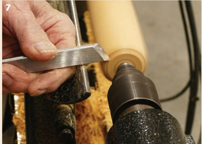
Trim the bottom of the handle with a skew chisel or spindle gouge.
