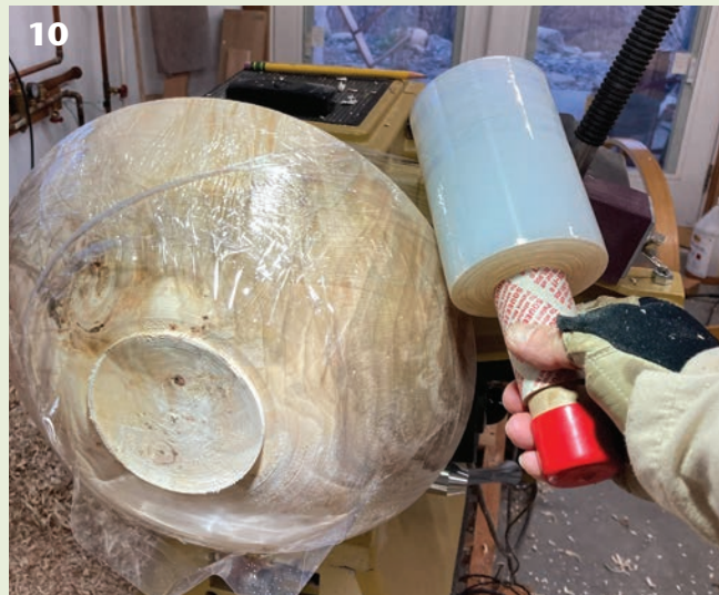
Stretch-wrap inhibits moisture exchange. It's best use is to prevent too much water from leaving a green blank as you work to hollow the interior.
