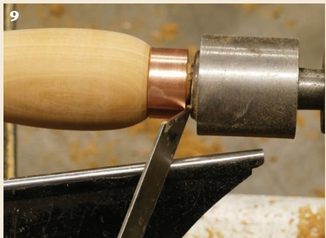
With the ferrule seated, trim the front edge with a narrow scraping tool.
