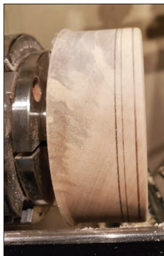
4, 5. Mark the total pendant depth on the side of the blank (left-most line) and round the side into a bead, as shown below.
