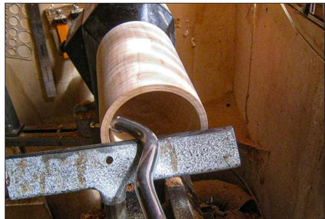
4. Use a deep hollowing tool to clean up the interior, much of which lies beyond the safe reach of a standard scraper.
