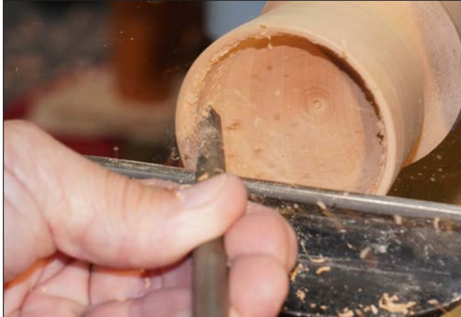
6, 7. I use the flat cutter presented at about 45° to the wood, rotating to near-vertical as I approach the sidewall. This shear-scraping cut leaves a refined surface that will need little sanding.
