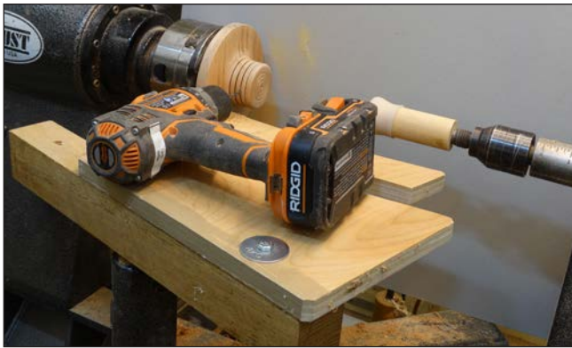
17. An adjustable-height shopmade platform aligns the drill bit with the axis of rotation.
