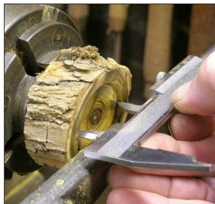
8. Transfer the diameter of the base's collar to the bottom of the lid.
