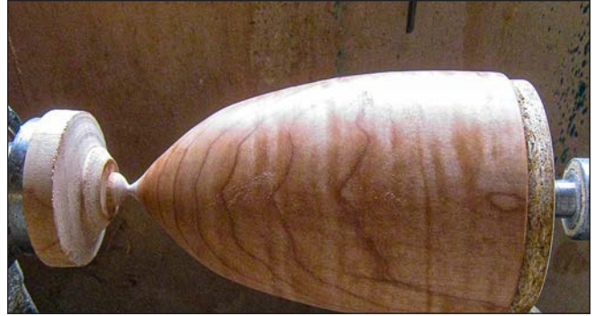
6. Shape the exterior, but leave the form attached with a small spigot for support.
