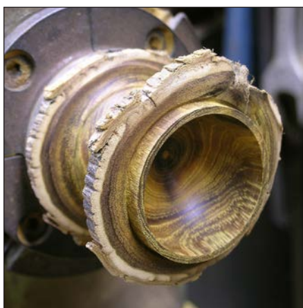
6. Hollow the interior using a small bowl gouge or round-nosed scraper. Use the outside of the form as a guide.
