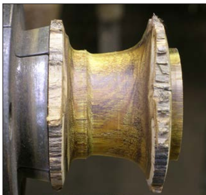
4. Begin shaping the base's exterior with a spindle gouge.
