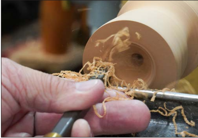
5. Hollow the interior using a series of straight-in push cuts, working your way from the center outward.
