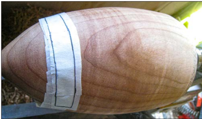
7, 8. Mark the slot for the phone on masking tape. This will guide the saw cut and reduce splintering. Clean up the bottom of the slot with a narrow bench chisel.
