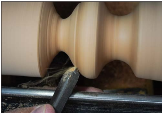
10. Shape the knob, continuing to work with the angled cutter as a scraper, then as a shear-scraper to refine the surface. Leave enough waste wood to support the blank through the sanding step.
