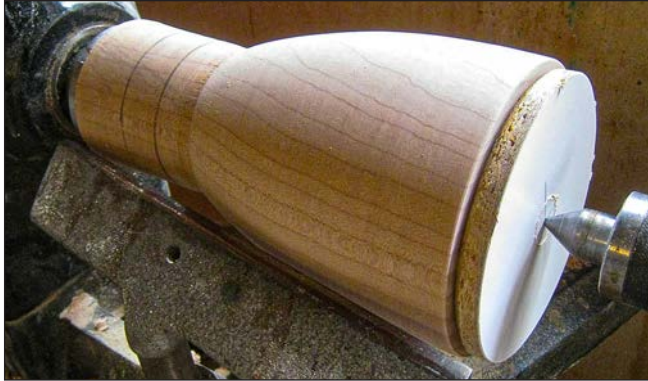
5. An insert turned from scrap lumber allows you to bring the tailstock up for extra support.
