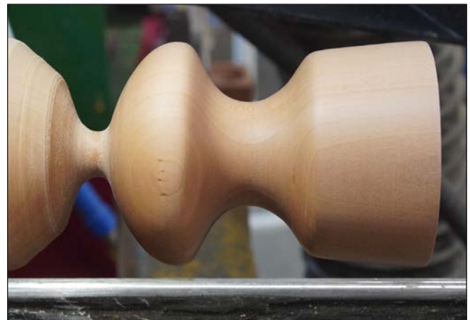
11. With the shape refined, sand the form and part it off.
