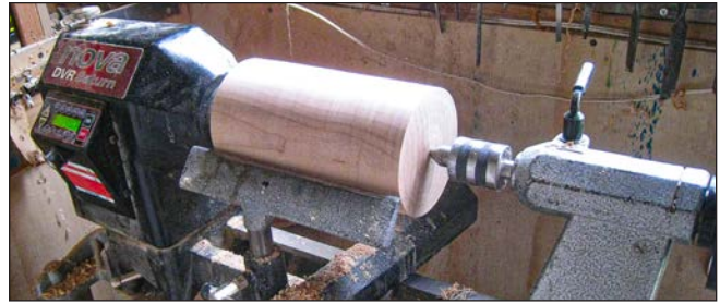
2. Mount the blank and round it using a spindle roughing gouge.
