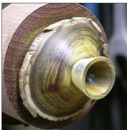
7. Hollowing the base enhances the delicate feel of the box.
