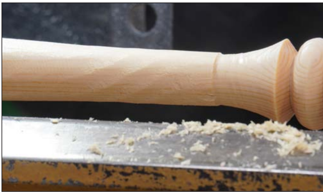
Photo 5. Chatter appears as the stock becomes thinner and the cut is farthest from tail- and headstock support.
