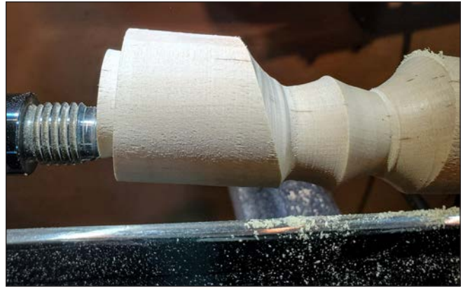
Photo 3. Turn the secondary axis base for the mushroom. Make sure to remove material until you are cutting wood continuously around the new axis.
