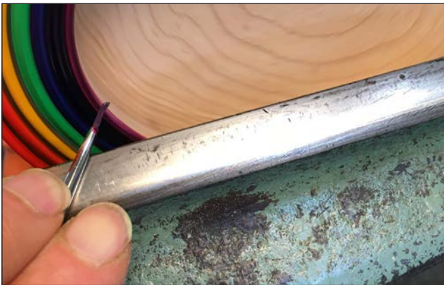
Photo 14. Wrap the last color (violet) into the bowl, aiming for a clean line where the paint ends.
