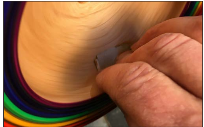
Photo 15. Carefully wet sand the undercut rim using the finishing oil as a lubricant; avoid sanding into the paint.
