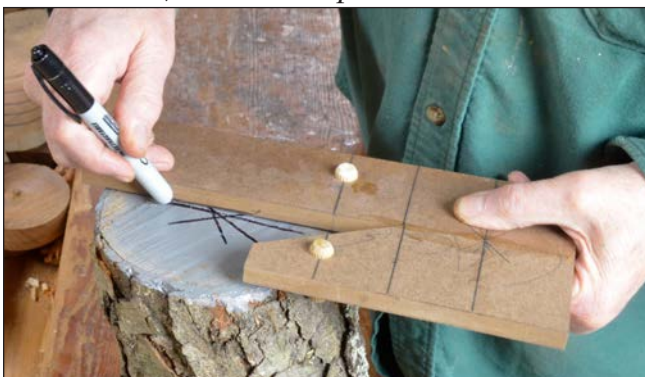
Photo 2. Bill of materials: MDF 1/2" × 2-1/2" × 11" and 2-1/2" × 6" cut 30°, two 1/2" dowels spaced 2-3/4" apart, #0 joinery biscuit.
