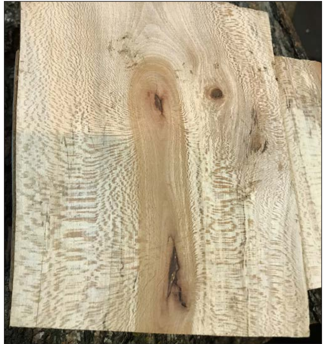
Sycamore in cross-section (above) and slabbed (right). Note the characteristic ray flecks in the piece at right.
