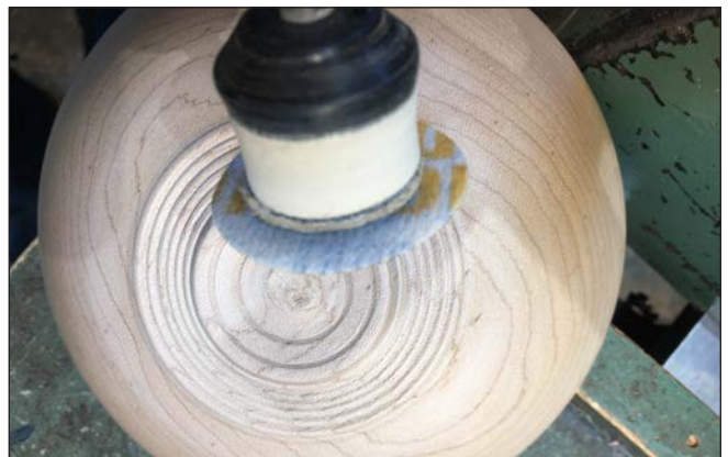
Photos 18, 19. Remove the nub from the base with a burr grinder or carving tool and sand away any tool marks.
