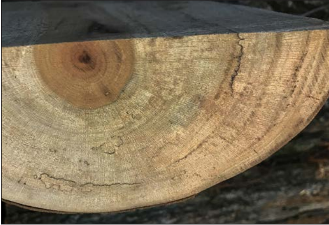
Sycamore in cross-section (above) and slabbed (right). Note the characteristic ray flecks in the piece at right.
