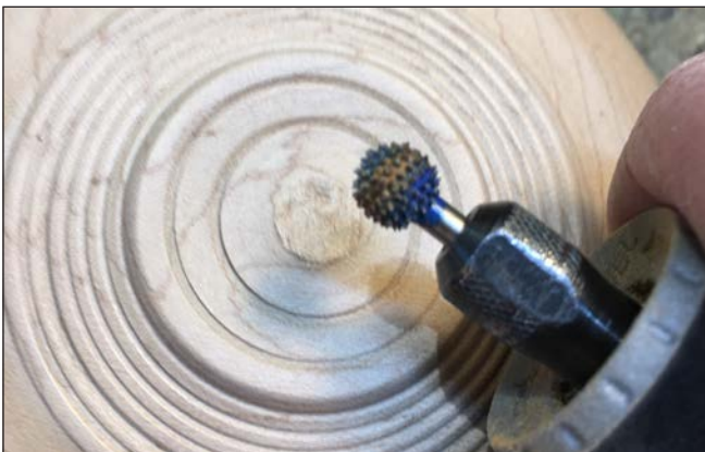
Photos 18, 19. Remove the nub from the base with a burr grinder or carving tool and sand away any tool marks.
