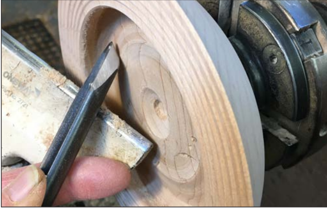
Photos 5, 6. Undercut the rim using either the detail gouge or round-nose scraper.
