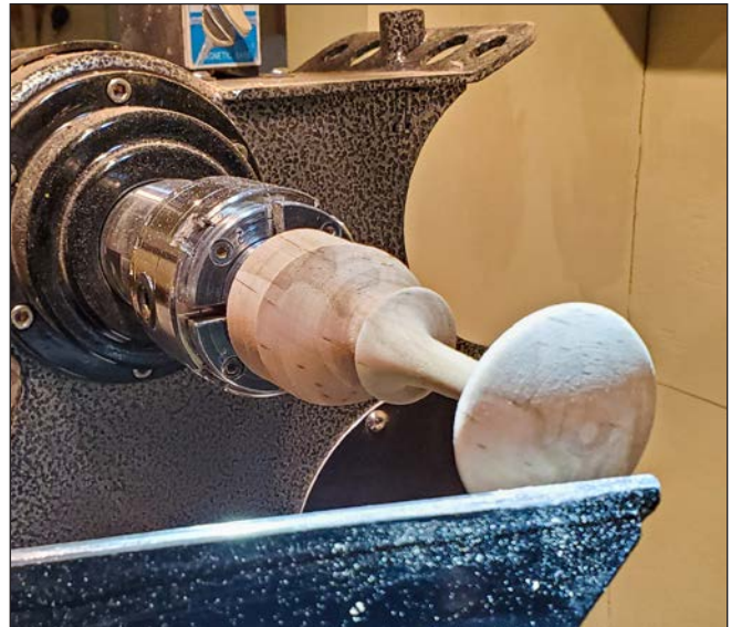
Photo 5. Remove the tailstock to complete the top of the mushroom. Sand the entire form using a light touch.
