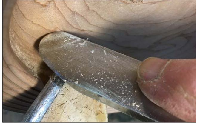
Photos 5, 6. Undercut the rim using either the detail gouge or round-nose scraper.
