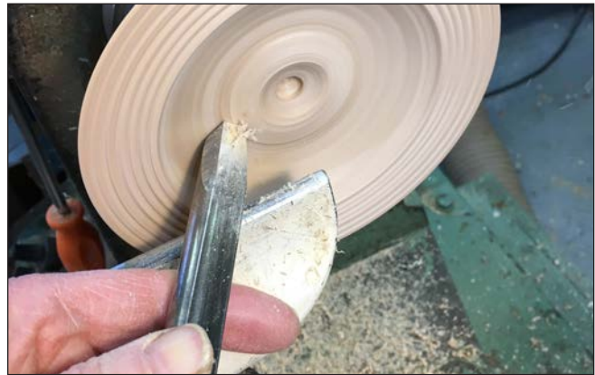
Photo 4. Start hollowing the form until you have room to undercut the rim.
