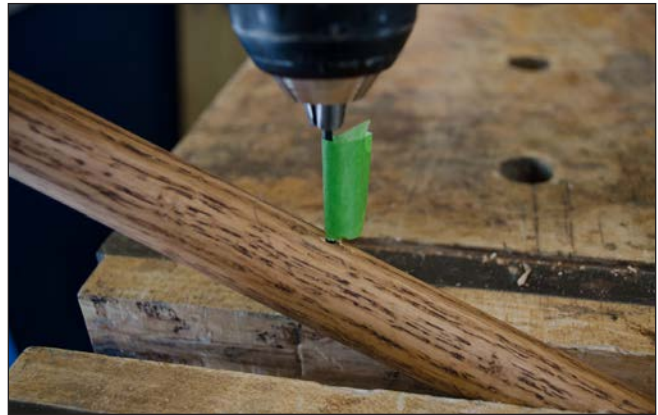
5. Drill for the toothpick dowels. The tape on the drill bit indicates hole depth.
