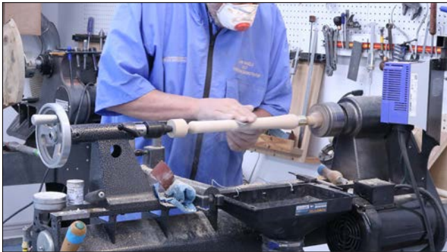
13. Sand the handle to remove tool marks. The wood should retain enough texture to assure a secure grip; 180 or 220 grit should do it.
