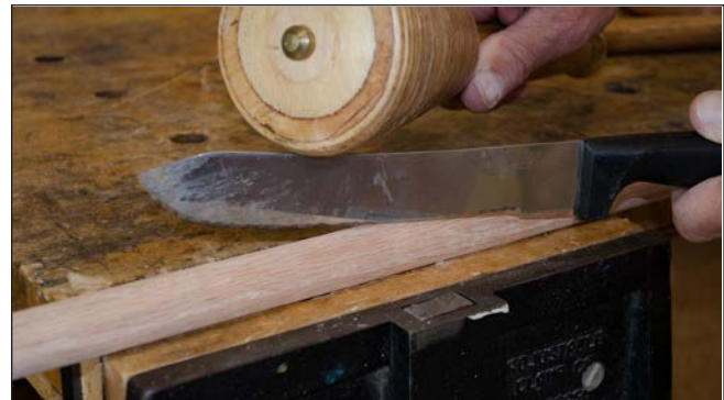
6. Split the paper joint with a dull knife and mallet.
