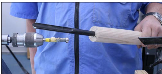
5. Test fit the steel before shaping the handle.
