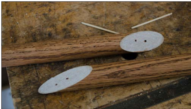
7. Clean the remnants of the paper and glue from the separated joint using white vinegar and scraping.
