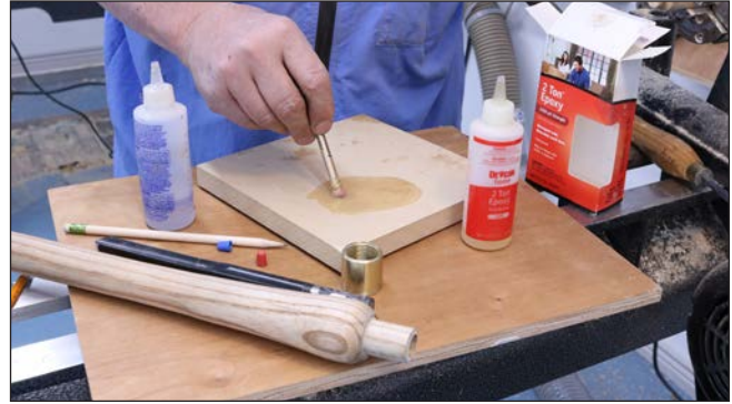
14. Secure the tool steel and ferrule with a two-part epoxy. Two-ton epoxy offers adequate open time and a strong bond.
