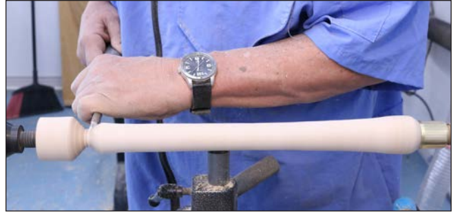
12. Shape the end of the handle with a spindle gouge.
