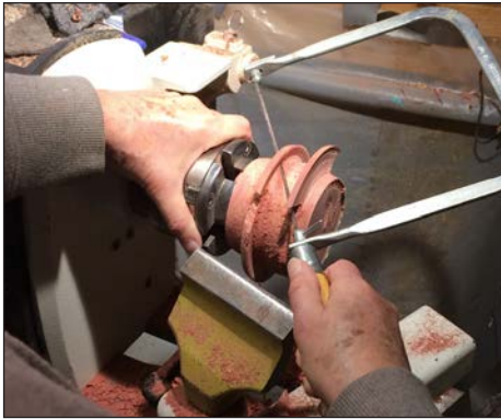
4. Use a coping saw to trim out waste in tight spots.
