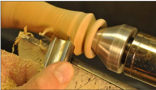
13. Cut in a downhill direction to go with the grain of the wood.
