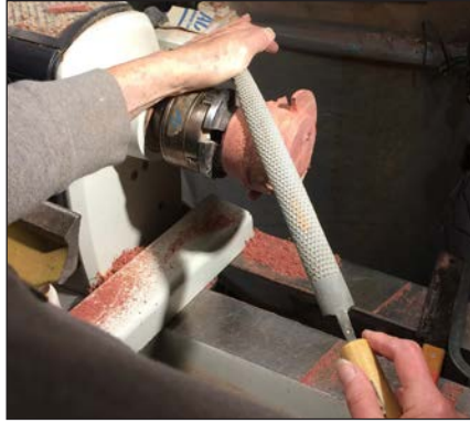
5. A rasp can remove a lot of waste quickly and can be used to add texture.
