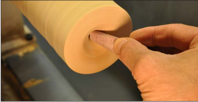
6. Shape the vase opening with a sharp bowl gouge and light cuts, then sand.
