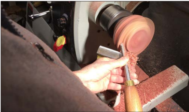
2. Take gentle cuts with a spindle gouge to form a curved surface on the fungi rings.
