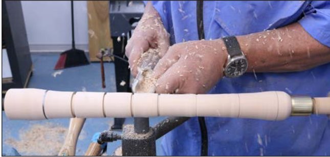
11. Reduce the blank to the set dimensions with a roughing gouge.
