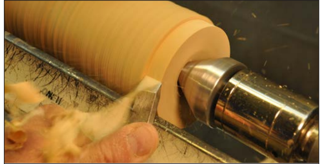
7. A peeling cut is useful for removing material quickly.
