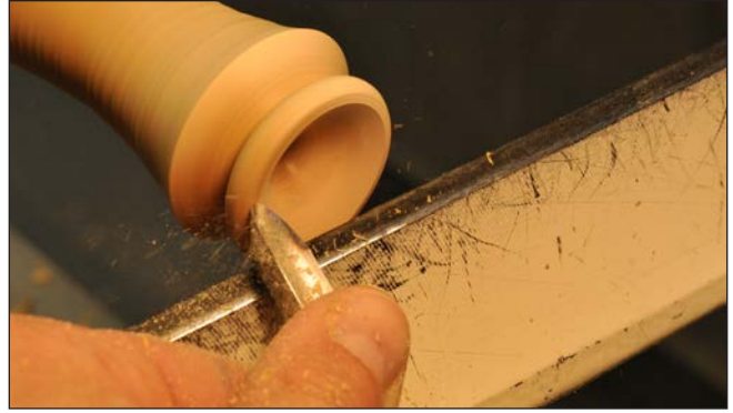
12. Refine the opening of the vase using light cuts.
