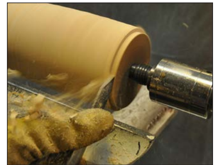
2. Use a parting tool to form a tenon to fit your chuck.
