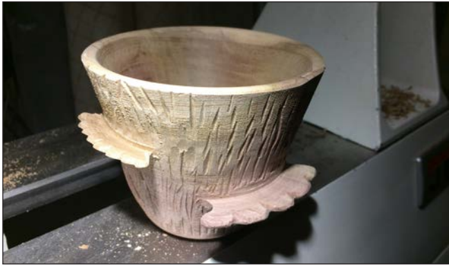
7. A powered carver efficiently adds realistic textures to the vessel's exterior.
