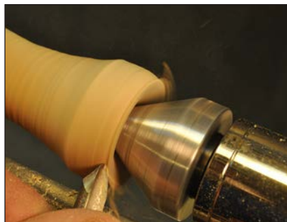
8-10. Form a bead at the top of the vase. A revolving cone center makes it easy to turn and blend the bead down into the hole.
