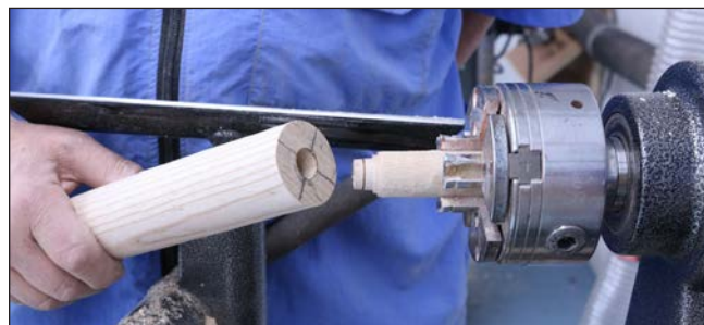
6. A shopmade friction drive turns the blank.
