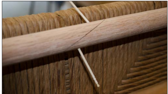
8. Test fit the spindle, using toothpicks to temporarily hold the scarf joint.
