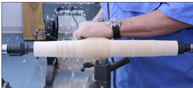
3. Work from the center out towards either end of the blank.
