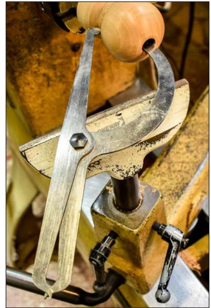
**7. Measure** — With the caliper points touching the wood inside and out, the free end shows thickness. Make hardwood about 1/8" (3mm) thick; light-weight woods can be thicker.
