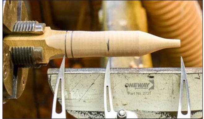
**11. Finial blank** — *Choose dry, straight-grain, knot-free wood, big enough once it's rounded to cover the flats on the ball. Stick with the rule of thirds to design the finial elements and details. Mark the mounting tenon and major divisions on the wood.*
