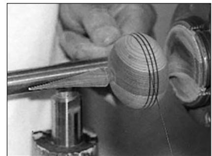
**6. Disguise the join** with lines burned by a stainless steel wire.
