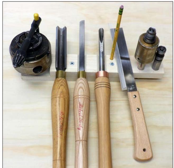
**1. Tools** — From left, scroll chuck, 3/4" (20mm) spindle roughing gouge, 1/2" (12mm) skew, 3/8" (10mm) bowl gouge, froe for splitting straight-grained spindle blank from sawn hardwood board, live center, and drive center.
