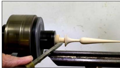
**16. Cut a tenon —** Sand the finial to 400 grit and apply a finish while it is on the lathe. Cut a  $\frac{3}{8}$ " tenon behind the bottom of the cove. Part off the finial.
