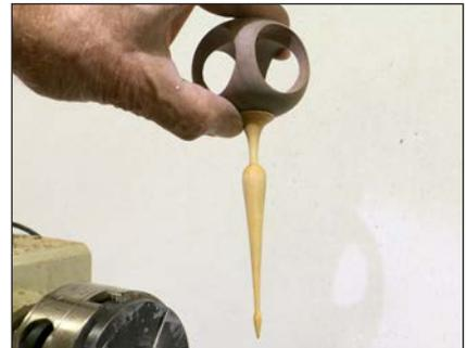
**17. Check the fit —** The tenon should fit the  $\frac{3}{8}$ " hole drilled in the cube.
