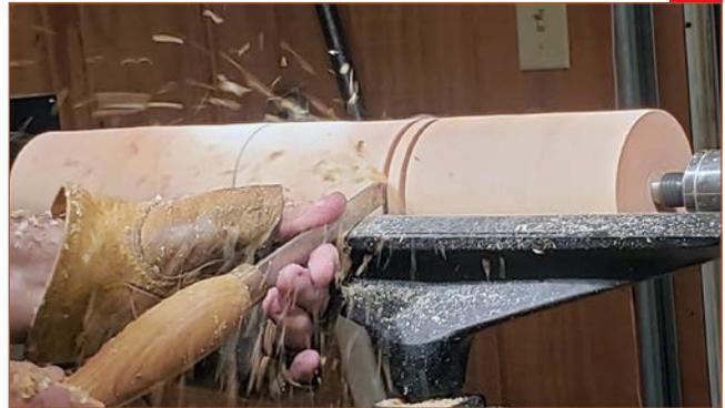
**5. Parting.** Grooves cut alongside the hat brim indicate final turning depth.
