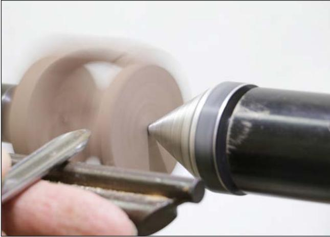
**5. Round the corners** — *The blank is small and you will be cutting air a good part of the time, so a lathe speed of at least 1200 rpm improves the cut surface. Round off the corners to make a sphere using a 3/8" (10mm) spindle gouge.*
