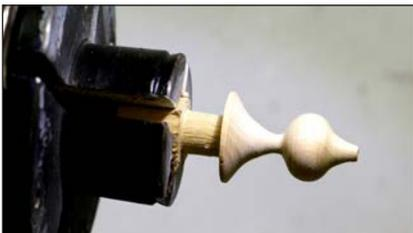
**18. Top finial —** Make a second finial for the top of the ornament, again making a  $\frac{3}{8}$ " tenon to fit into the hole in the top of the cube. This finial is about 1"- (25mm-) long. Sand and finish the finial on the lathe.
