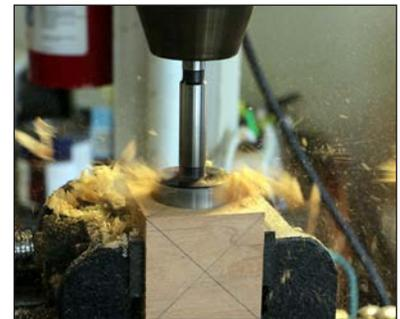
A drill press offers an alternative to boring on the lathe. Secure the blank in something other than your hand.
