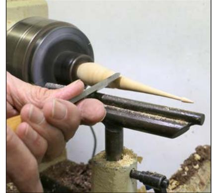
**14. Shape the "onion"—** Smooth the long transition from the tip, then shape a bulb. Finials are developed by completing elements from tail end-to-headstock.
