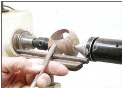
**7. Rub the bevel** — *Start the cut with the bevel on the wood. Check tool presentation with the lathe off and you will be less likely to get a catch.*
