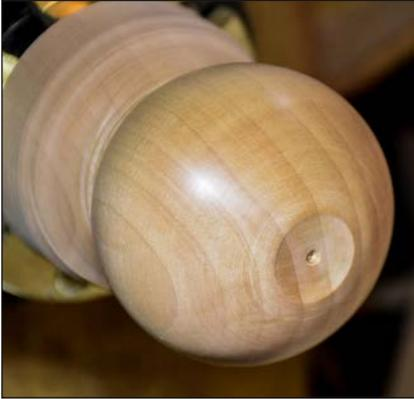
**4. Bore** using a 1/2" (12mm) bit in the tailstock chuck. Slow the speed down, clear the chips frequently, and hold the chuck when withdrawing. Bore through the ball into the tenon, beyond the bottom of the globe.
