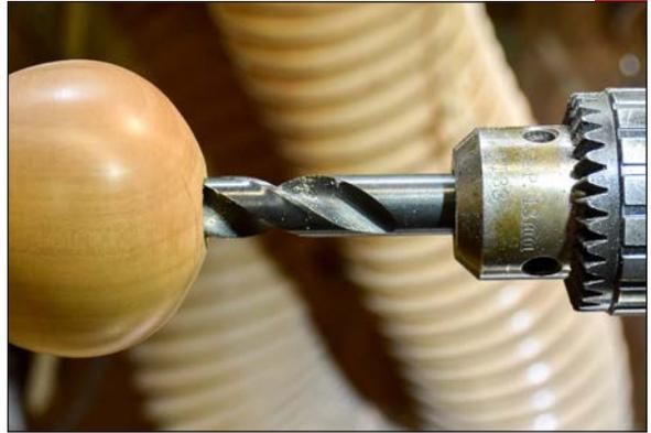
**3. Flat** — Make a flat spot for the finial, much easier than trying to fit it to the curve of the globe. Cut a dimple to give the drill bit a start.
