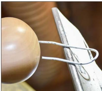
**8. Wire gauge** — With one end bearing on the inside, the free end indicates thickness without scratching the outside.
