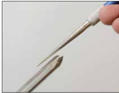
7 Hone flute. Conical fish-hook sharpener removes burr from inside the flute.
