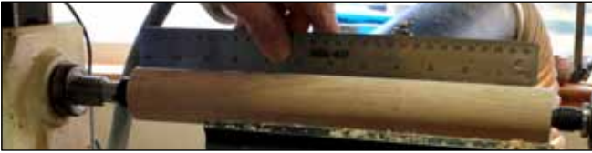
7 Check the diameter of the roller with a vernier caliper, and its flatness with a straightedge.
