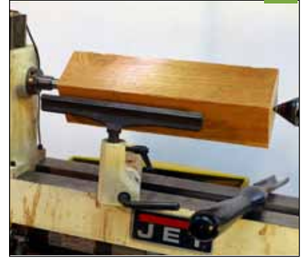
4 Spindle turning - the grain of the wood runs parallel to the lathe axis.
