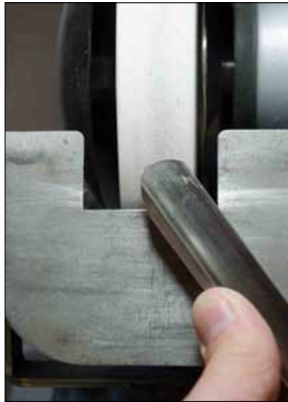
4 Sharpening. Swing the handle right while rotating the flute.
