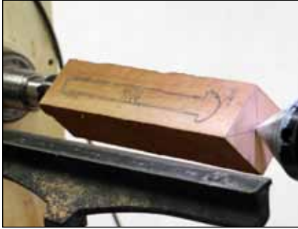
15 Sketch the pin on the blank; there's plenty of extra wood.
