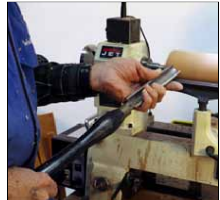
5 (left) Stand easy and brace the gouge handle on your body. Lift the handle to cut.
