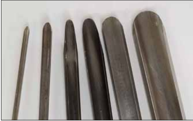
1 Spindle gouges. The fingernail shape is characteristic, with a finer, more pointed tip for detail work.
