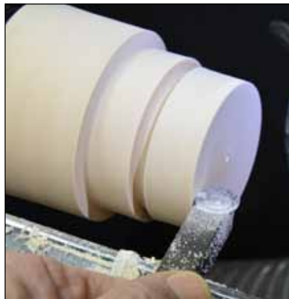
11 The carbide-tipped half-round scraper makes a smooth surface on endgrain.
