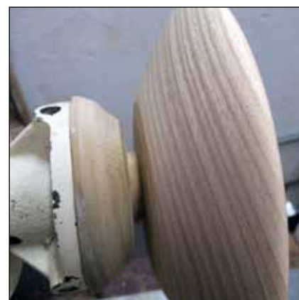
2 The bowl is mounted on a glueblock for turning the inside. Reducing the thick glue block to a small tenon allows tool access to most of the bowl's body.
