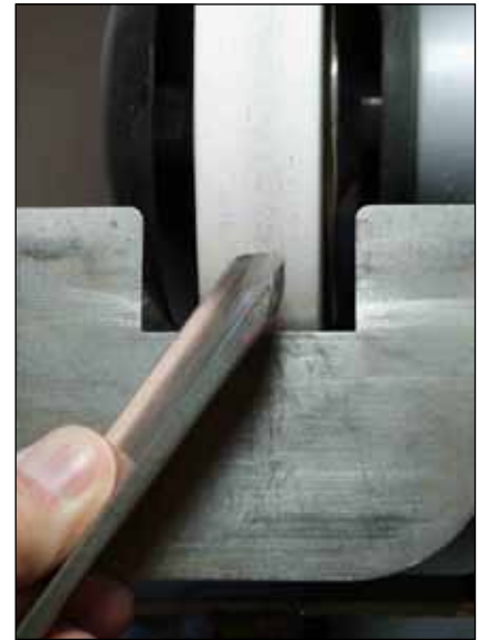
5 Sharpening. Swing left while rotating the flute.
