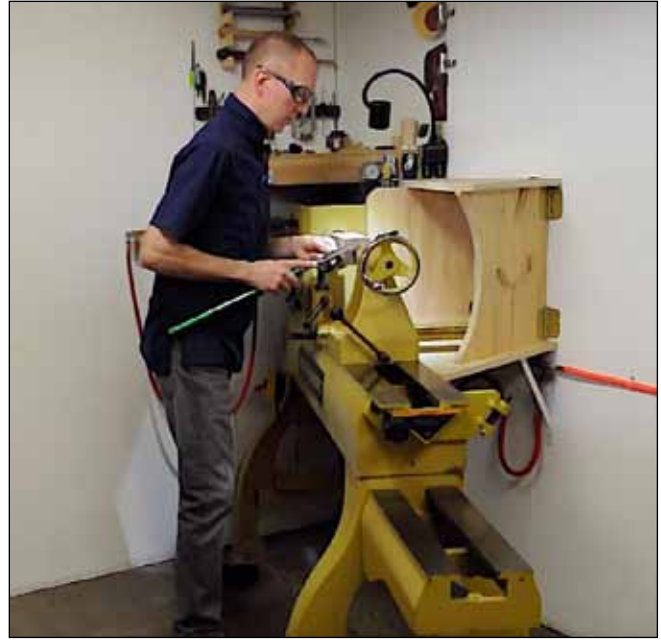
5, 6 Squatting and extending your legs, with the tool an extension of your body, controls the tool's cutting edge.
