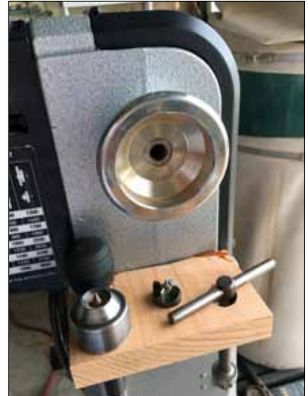
Epoxy holds wood tool shelf on end of midi lathe. .
