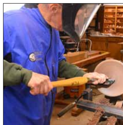
15 Bevel. To keep the bevel gliding, raise the handle of the gouge as you arc toward center.
