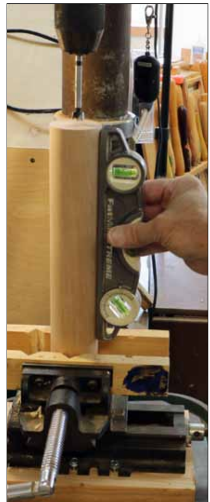
9 A vise holds the roller on the drill press table; the level checks for vertical alignment.
