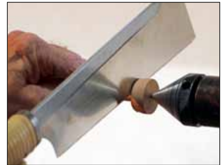
21 Saw through the neck to remove the pin from the lathe.
