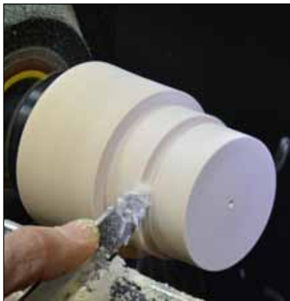
10 Part a shallow groove to limit the first face.
