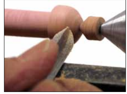
20 rotate the flute on the curve to take fine cuts, leaving a neck.
