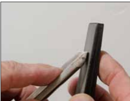
6 Hone bevel. Stroke it on a 600-grit diamond plate.
