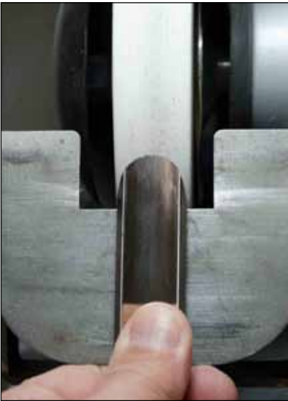
3 Sharpening. Start in the center with the flute facing up.
