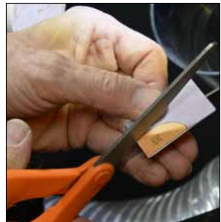
18 Print out the full-size template onto heavy paper or file card, fold it in half for symmetry, and cut it out.
