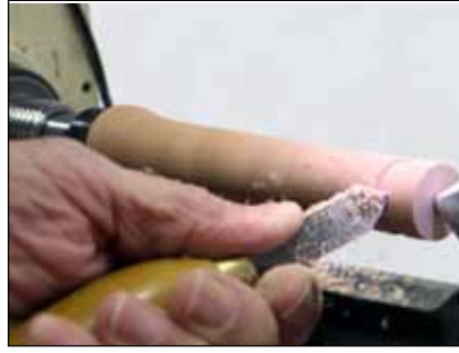
16 The parting tool makes a shoulder to define the head of the pin, with extra for clearance.
