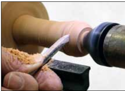
13 Reverse the blank and use the spindle gouge to shape the wood.
