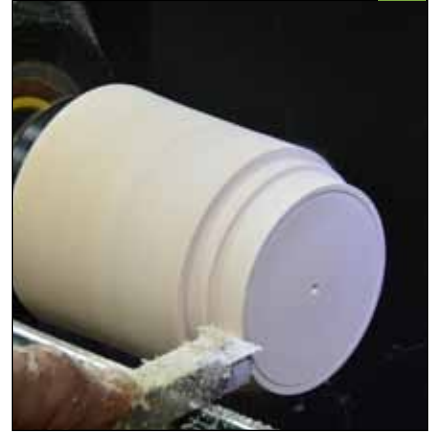
9 A carbide-tipped scraper also leaves a clean, smooth surface.
