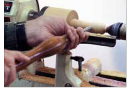
14 Aim the gouge bevel in the direction you want to cut.
