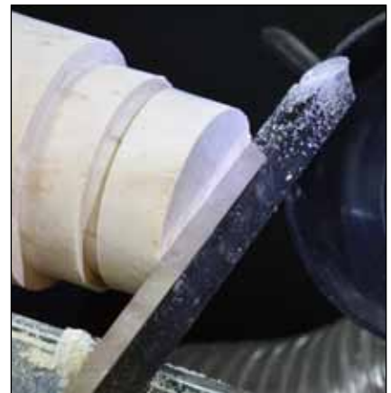
12 Use the straight part of the tool to check the end for flatness.
