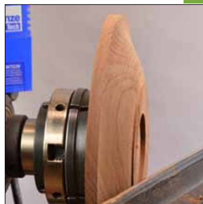
12 Chucking recess and plate back. The bowl gouge and scraper teased out the plate's ogee profile.
