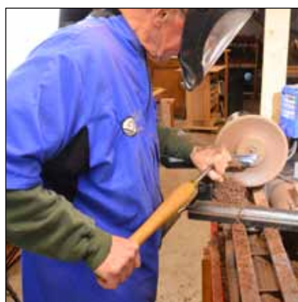
14 Hollow the plate with the bowl gouge. Aim the flute in the direction you want to cut, with the bevel skimming the just-cut wood.
