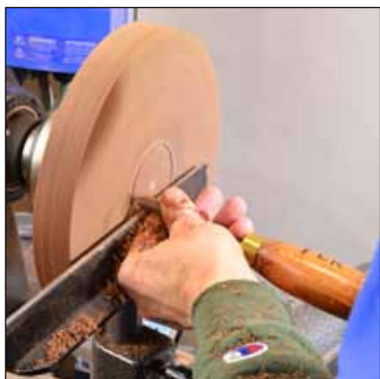
10 Groove to start the chucking recess, with the parting tool.
