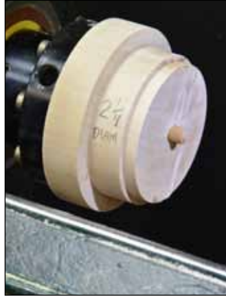
14 Bore the chuck for a short dowel.
