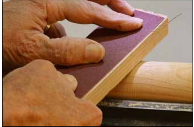
8 Remove tool marks with a sanding stick made by gluing sandpaper to a flat board.
