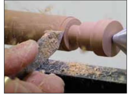
17 Rough the pin to round then bring it down to final diameter with the parting tool.
