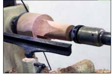
12 Mount the handle between centers and turn toward the tailstock as far as possible.
