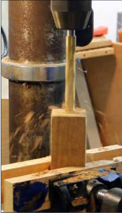
10 Use the drill press to bore through the handle blanks.
