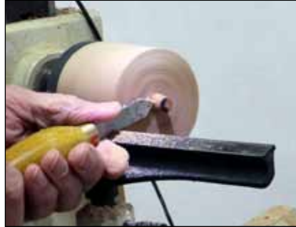
11 Jam chuck. Mount it on a faceplate and turn a centering nub.
