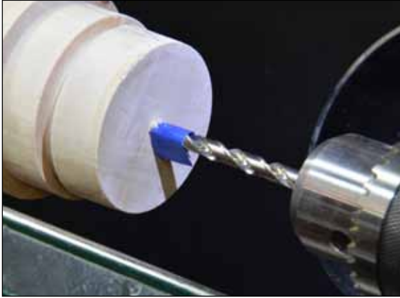
13 Tape flag indicates the depth of the hole. Boring on the lathe is very accurate.
