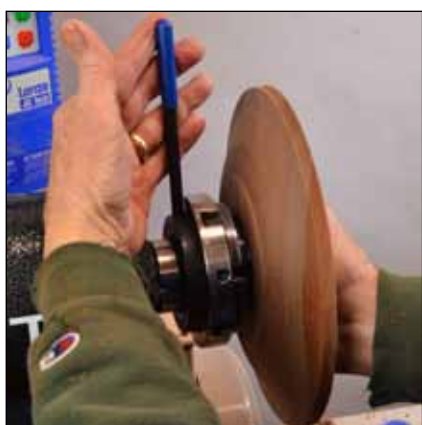
13 Expand the scroll chuck into the chucking recess. The right-sized recess matches the nearest-to-circular setting of the chuck jaws.
