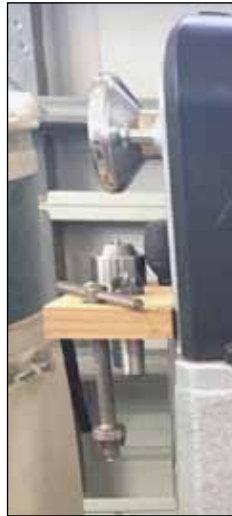
Epoxy holds wood tool shelf on end of midi lathe. .
