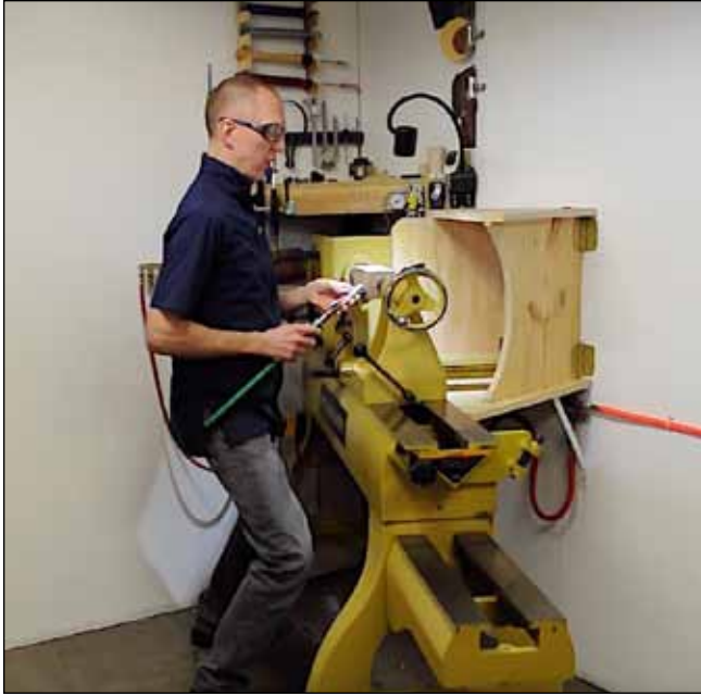
5, 6 Squatting and extending your legs, with the tool an extension of your body, controls the tool's cutting edge.
