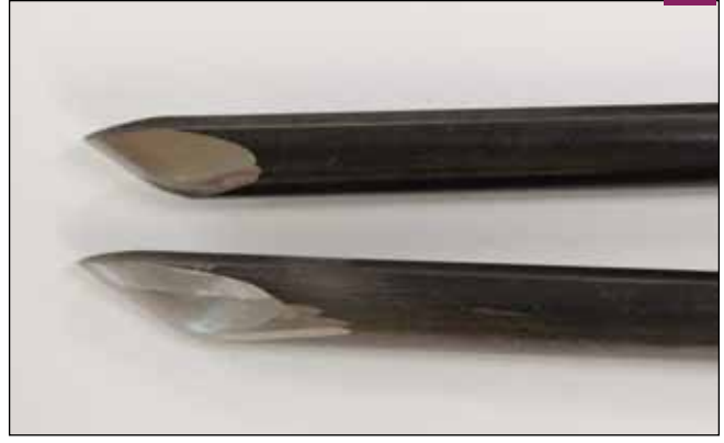
2 Bevel angle. Top, 35° bevel, with rounded heel. Bottom, short 35° bevel with three secondary bevels.
