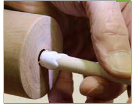
24 Use a small dowel to spread waterproof glue inside the hole.
