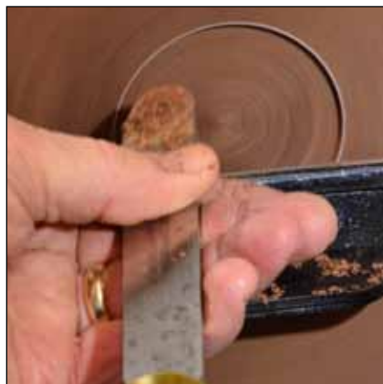
11 Excavate with the bowl gouge and heavy scraper.
