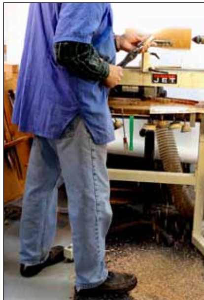
5 (left) Stand easy and brace the gouge handle on your body. Lift the handle to cut.
