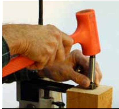
3 Center and tap the drive spur into the end of the workpiece.
