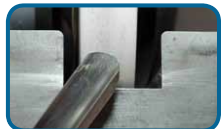
7 Hone flute. Conical fish-hook sharpener removes burr from inside the flute.
