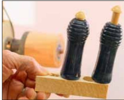
23 Polyurethane varnish dries on the dyed handles.
