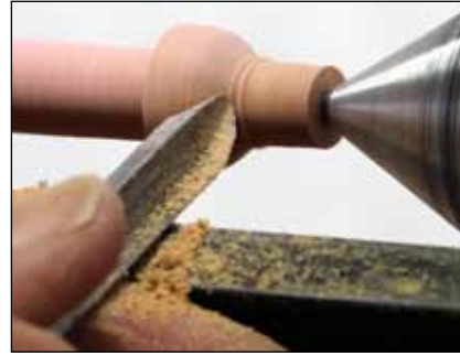
19 The spindle gouge forms the head of the pin.
