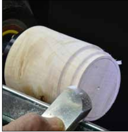
8 The skew chisel peels the wood away. With the bevel rubbing, raise the handle to cut.
