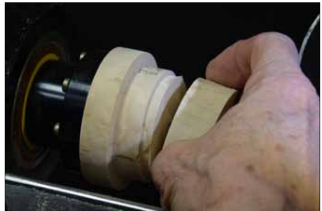
16 Press the yo-yo side blank onto the chuck.
