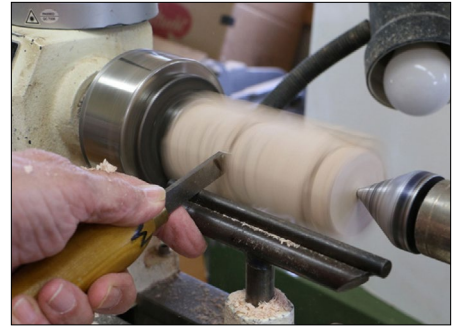
Photo 5 - Defining the ends of the egg with a parting tool.
