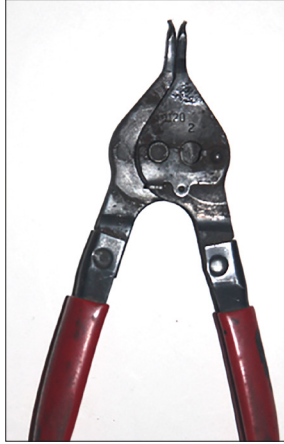
Snap Ring Pliers exert pressure in the expansion and compression mode. The pliers make holding the brass tubes and inserting them into pen blanks a lot less messy.
