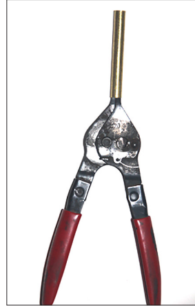
Snap Ring Pliers exert pressure in the expansion and compression mode. The pliers make holding the brass tubes and inserting them into pen blanks a lot less messy.
