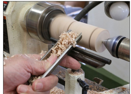
Photo 6 - Roughing to round and final diameter with a spindle roughing gouge.
