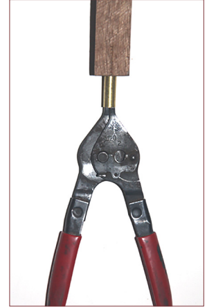
Snap Ring Pliers exert pressure in the expansion and compression mode. The pliers make holding the brass tubes and inserting them into pen blanks a lot less messy.
