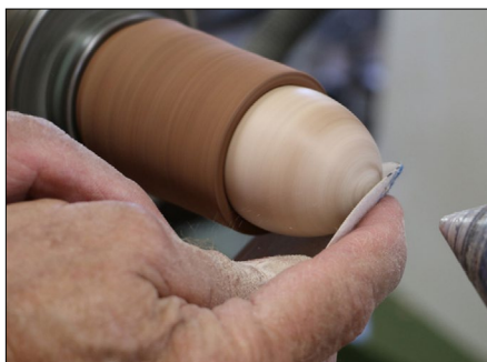
Photo 23 - Sanding the egg in a jam chuck.
