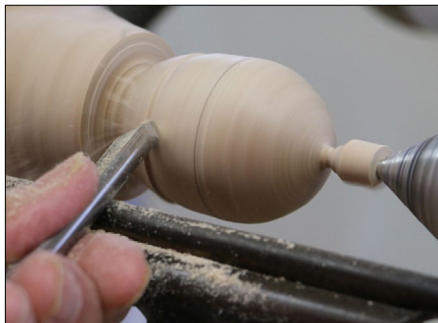
Photo 14 - Shaping the pointy side.
