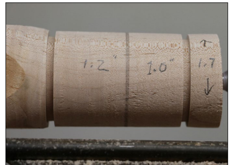
Photo 7 - Redrawing the location of the largest diameter.
