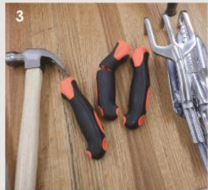
2 How you remove the stock handles depends on the set you acquire. The author used a coping saw for the first effort before realizing the rubber handles were simply pressure fit on this set. A hammer and scrap block of dimensioned lumber made quick work of the second and third handle removals.
