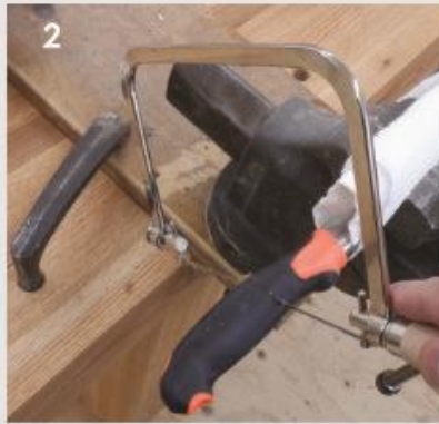
2 How you remove the stock handles depends on the set you acquire. The author used a coping saw for the first effort before realizing the rubber handles were simply pressure fit on this set. A hammer and scrap block of dimensioned lumber made quick work of the second and third handle removals.
