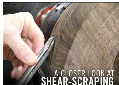
Shear-scraping with the edge of a shear scrape on an olive wood bowl. The shear scrape is held at an angle to the wood and with the cutting edge parallel to a steep angle.
