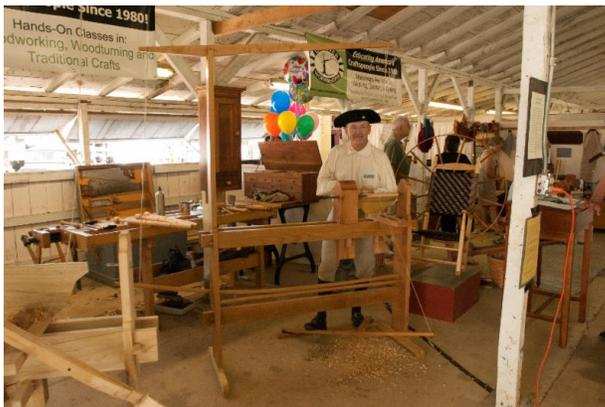
*Ernie modified plans given to him by Roy Underhill for this spring-pole lathe, sizing it to modern stature. The outboard poppet (tailstock) is a solid piece of cherry. His apprentice at the time also made one and they built stools at the county fair. The two lathes working together drew huge crowds.*
