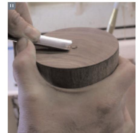
The first set of centers positions the wood at a significant angle on the lathe. It is actually quite balanced, but as the turning progresses, it becomes less balanced, sometimes requiring the lathe speed to be adjusted. Before changing centers, I sand the work (6, 7).
