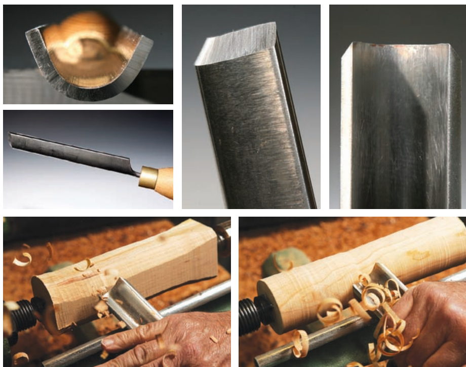
a spindle-roughing gouge (SrG) is used to turn a square spindle into a cylinder.
