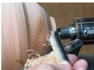
A pull cut is used to reach into a tight area and to clean up torn grain. For an even finer shear-scraping cut, rotate the tool slightly clockwise and drop the handle.
