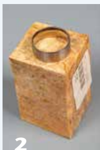
2 Stabilized burl is a good choice, as it won't move much with humidity changes. Size the wood so there will be enough thickness all around the ring core, then cut off a slice slightly wider than the height of the ring core.
