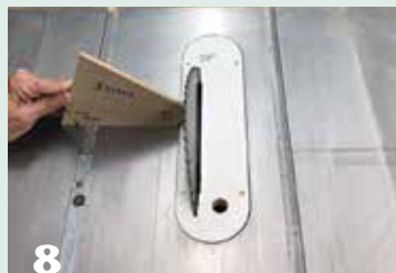
8 A single set-up wedge is used for both blade and fence angles. Set the blade angle using the small end of the set-up wedge.
