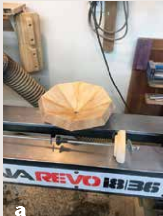
a A simple shopmade drawbar comprises all-thread rod and a centering cone.
