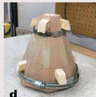
d For deeper bowls, the glue blocks just keep the hose clamps from sliding up the tapered sides.
