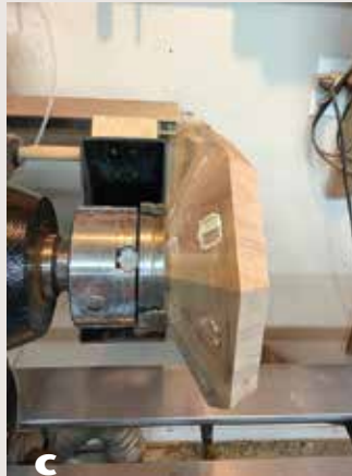
c The small end of the workpiece sits on the flats of the four-jaw chuck, while the drawbar centers and holds the workpiece firmly.
