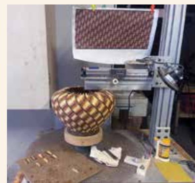
A horizontal assembly jig, originally developed by Ray Feltz and subsequently enhanced by Tom Lohman, accurately places thousands of segments. This version of the jig was designed in 2018.
