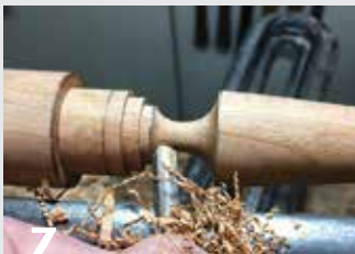
6 A central line indicates the left edge of the cove and the right edge of an angled cut, which is formed with a skew.
