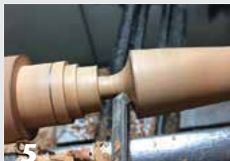
5 A spindle gouge is used to shape the right half of the cove under the blade.
