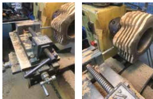
Deep, straight-in cuts made with a machine tool bit held in a vise highlight the log's irregular outer surface.
