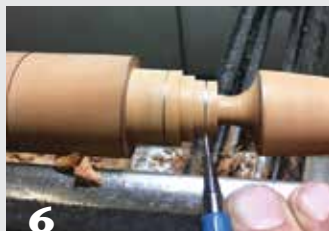
6 A central line indicates the left edge of the cove and the right edge of an angled cut, which is formed with a skew.
