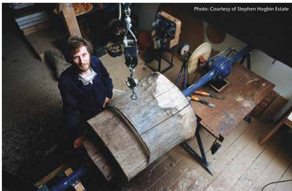
(Left) Stephen Hogbin was always pushing the envelope, pictured here with his truck-axle lathe, 1978. For stability when working with huge pieces of wood, the lathe was attached to the building by lally column at the tailstock and bolted to the floor joists at the headstock.
