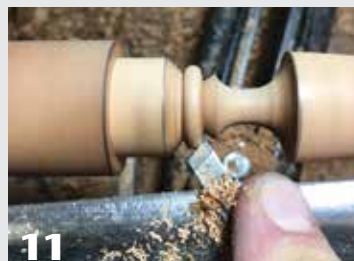
Left of the angled cut is a central bead. A central pencil mark aids in shaping first one side, then the other. The author uses a small skew, presented on its side as a scraper, to shape the bead.
