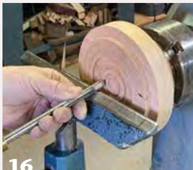
16 The author forms a chucking recess and adds beads to decorate the inside of the box lid.
