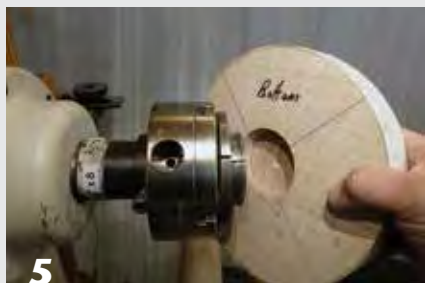
5 Mount the lamp base on your chuck by expanding the jaws into the hole on the bottom.
