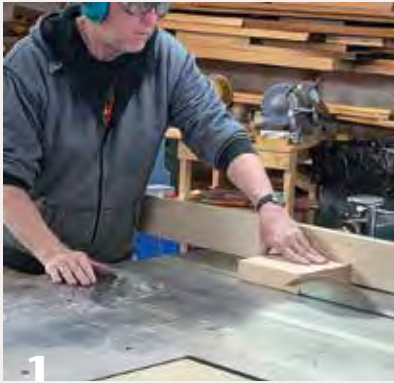
1 The author prepares box blanks by cutting squares on the table saw. Tilting the blade to 9 degrees creates an elegant bevel.
