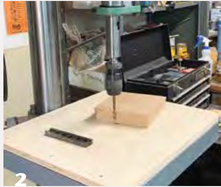
2 Predrill the blank so it can be threaded onto a screw chuck. The pilot hole doubles as a depth indicator for hollowing.
