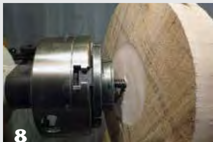
8 Mount the top of the base onto the screw chuck. The chuck jaws will register against the turned flat area.
