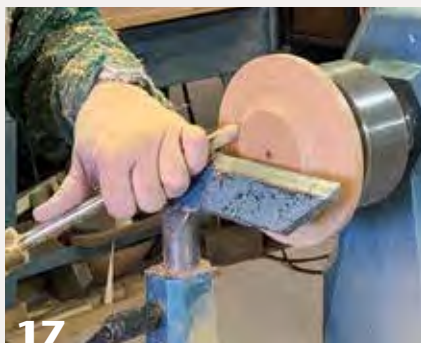
17 With the lid now mounted in a chuck in expansion mode, the author turns and sands the top of the lid.
