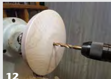
12 Enlarge the center hole with a \frac{1\frac{1}{32}} " or \frac{7}{16} " twist drill to fully accept the \frac{3}{8} " OD lamp rod.
