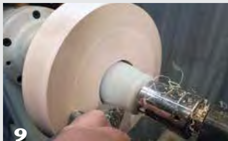
9 Use a bowl gouge and shear-scaper to turn the bottom of the lamp base. After truing up the outside edge, form a concave surface in the middle. A straightedge touching only the outer edges indicates concavity.
