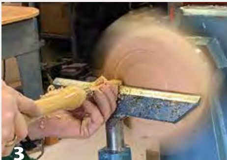
3 With the box mounted on a screw chuck, form a chucking recess in the bottom. Decorate and sand.
