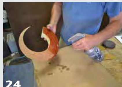
24 The author sprays the veneered form with a shellac/alcohol mixture, which reveals sanding marks and protects the surface during repair/touch-up.
