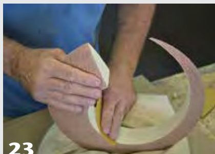
23 Sand carefully to avoid breaking through the thin veneer.
