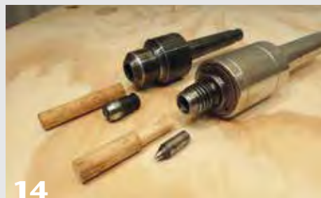
14 Two alternatives for mounting dowels in the tailstock live center with center point removed. Top: straight-walled live center with setscrew. Bottom: tapered live center with no setscrew.
