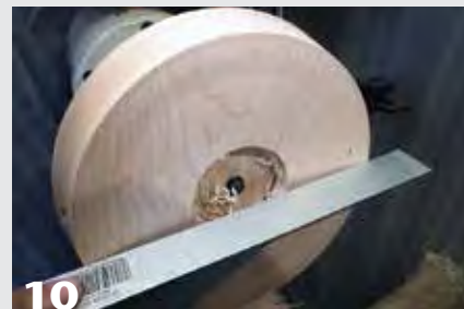
9 Use a bowl gouge and shear-scaper to turn the bottom of the lamp base. After truing up the outside edge, form a concave surface in the middle. A straightedge touching only the outer edges indicates concavity.
