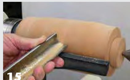
15 A spindle-roughing gouge is used to turn away the edges of the box.
