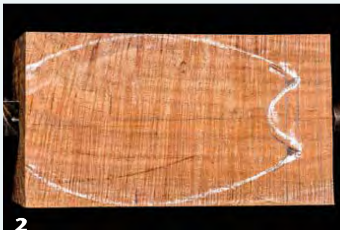
The intended vessel's outline chalked on the wood serves as a guide when roughing.
