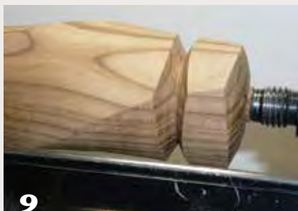
Turn the end of the twisted spindle to a slightly convex shape, and match that curve at the other end of the napkin ring.
