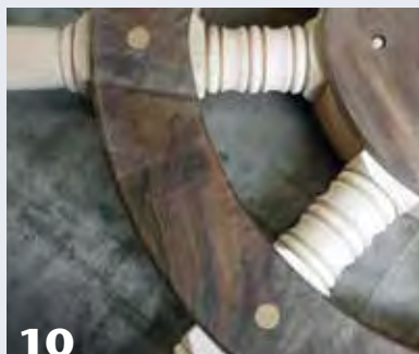
10 The turned spokes are inserted through the wheel and into the hub, then pegged in place. The hub pegs will be hidden by the fit-up clock.
