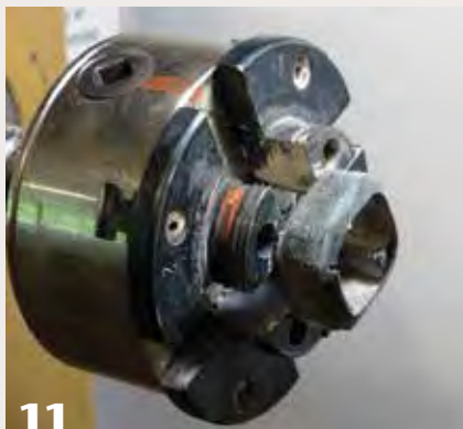
A length of bicycle inner tube fits over the chuck jaws to protect the napkin ring from being marred. Reverse-mount the napkin ring, using the chuck in expansion mode.
