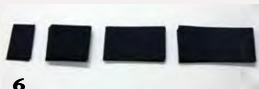
6 Cut veneer accent pieces slightly larger than needed and trim flush to the segments.
