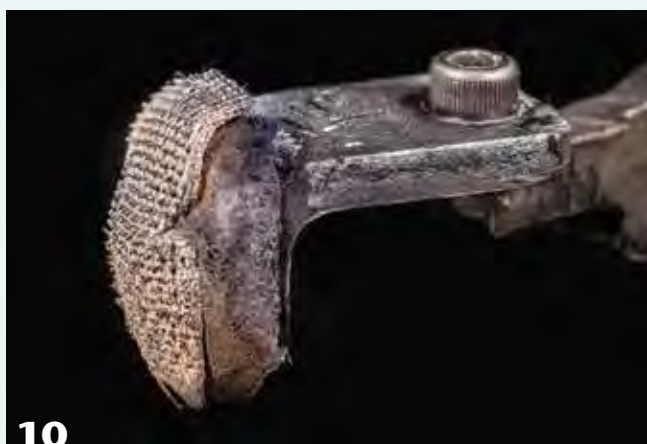
The author's shopmade sanding attachment, which mounts on his Stewart tool for reaching inside vessels. An angle of metal with hook-and-loop material glued onto it holds the abrasives.
