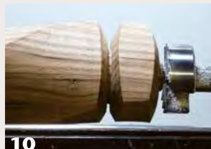
Drill through the napkin ring until it is cut free.
