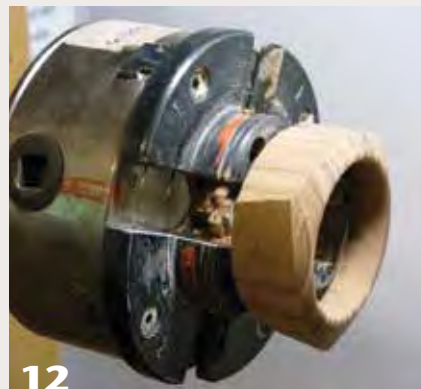
A length of bicycle inner tube fits over the chuck jaws to protect the napkin ring from being marred. Reverse-mount the napkin ring, using the chuck in expansion mode.
