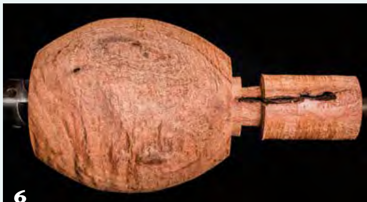
6 The “small bark inclusion” went far deeper than anticipated and was in fact an inner fault revealed during turning.
