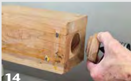
14 Position the tailstock plug you turned earlier to give the live center a surface to contact. Tailstock support will increase stability while shaping the vase.
