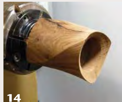
14 Use a Forstner bit to drill into the spindle deep enough to allow the tea light candle to sit all the way in and flush with the top.
