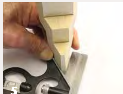
5 Confirm the accuracy of the 45-degree stave angle.
