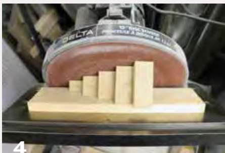
4 Ensure the bevels on the glued-up staves are smooth. As a safety measure to keep his fingers away from the abrasive disk, the author taped the test segment to a carrier board.
