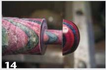
After the magnets are installed, the exposed hole on top of the box lid can be concealed with a decorative button of a contrasting wood species.
