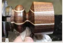
After sanding the piece, the author applies a light coat of mineral oil both inside and out. This project could just as easily have no finish at all, depending on your preference.
