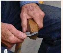
Slow the carving process down to whittling speed and it is easier to understand the interaction between a cutting edge and grain orientation. Even in slow motion, forcing the tool in the wrong direction will result in a catch.
