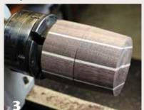
With the blank mounted in a four-jaw chuck, turn a slight taper from a line drawn 2" from the end.
