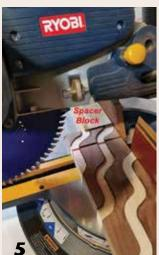
Precise joinery is critical to successful segmented forms. To cut the staves, set a miter saw to 60° with an angle gauge. A spacer block with a 60° bevel clamped to the fence ensures each stave is the same width. Flip the board between each cut.
