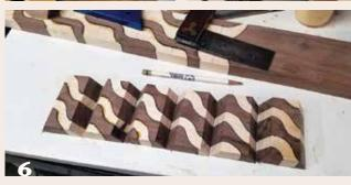
Lay out the cut staves in the order in which they were cut from the board.
