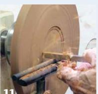
Re-chuck the blank and true the top, then widen the chucking recess to accommodate the cork insert.
