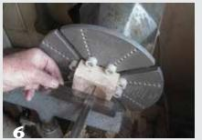
Use a depth gauge to ensure about  $\frac{1}{4}$ " thickness at the bottom.
