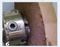
Remount the blank by expanding the chuck jaws into the recess in the top.
