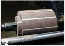
Mount the blank between centers and form a tenon that will fit in your chuck. The hole left by the point of the drive center will help align the blank when re-chucking later.
