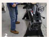
A wide stance with unlocked knees allows you to move your body—but not your feet—smoothly through the cut, guiding the tool around a flowing curve.
