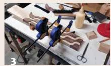
After checking the dry fit, insert a piece of contrasting veneer between each element before gluing and clamping the segmented elements together.
