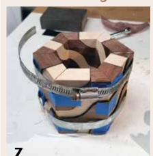
Assemble and glue the staves, filling two opposing joints with spacers and no adhesive. Clamp the assembly.
