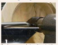
Bowl gouges are designed to cut at the centerline. Adjust the toolrest height and verify the cutting point of the tip of the horizontal tool aligns with the center of rotation.
