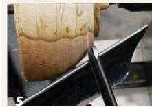
The tool's cutting tip should maintain a consistent relationship to the blank throughout the turn—unless you want a dip, high spot, or catch.
