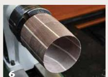
The author uses a freshly sharpened scraper to make final cuts to form the thin rim of the biscuit cutter. The interior walls near the rim are cut parallel to help ease biscuit removal during use; the tapered exterior walls provide added strength to this thin area.
