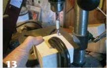
Clamp the box and lid together before drilling the magnet holes. One hole, drilled through the lid and into the box body, ensures perfect alignment.
