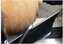
Too much cutting edge presented to the blank creates an aggressive, difficultto-control cut. This gives the wood the opportunity to pull the tip of the gouge into the rotating wood, causing a dramatic catch.
