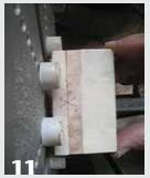
Scrape the underside of the lid to remove saw marks, then test for a good union by holding up the box.
