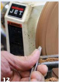
Decorate the rim with a suitably elegant profile. Remove the piece from the lathe, finish, and add the cork insert.
