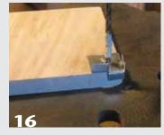
The author's shopmade drill guide template positions the hole location consistently, ensuring proper alignment of the catch magnets in the body and lid.
