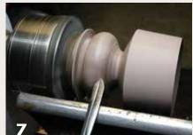
Form the upper section of the biscuit cutter, including a knob/handle to a shape of your liking.
