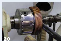
If your chuck and jaws will accommodate the task, an alternative is to reverse-chuck the wine caddy in expansion mode to access the bottom for turning and sanding.
