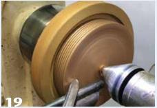
Make a jam chuck with a recess to fit the rim of the wine caddy (recess is colored red for clarity) and turn the caddy bottom, again slightly concave. Bring up the tailstock for all but the final cut to prevent the caddy from becoming a flying saucer.
