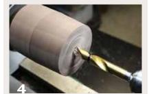
A hole drilled to a depth of 11/8" serves as a starting place for hollowing. Not pictured, a round-nose scraper does a nice job of hollowing endgrain, cutting from center toward the rim.
