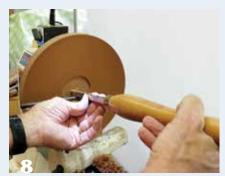
(7-8) True the rim and turn a recess in the bottom for re-chucking.
