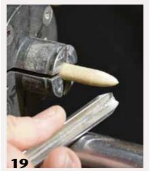
The bird's beak can be turned to a rounded or pointed end, or for a singing bird with the appearance of an open beak, saw a small wedge into the end of the blank. Glue the beak into the bird's head.
