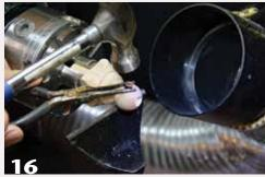
With the head still partially turned, mark eye location and drill holes to accept short segments of a colored pencil. Glue and tap in the pencil pieces, using the toolrest underneath for added support.
