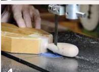
Mark and cut away the underside of the bird's body. Note the still-square head section is held securely in a wooden handscrew clamp for safe bandsawing.
