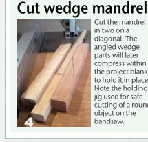
Cut the mandrel in two on a diagonal. The angled wedge parts will later compress within the project blank to hold it in place. Note the holding jig used for safe cutting of a round object on the bandsaw.
