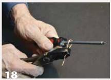
The copper core of 12-gauge electrical wire, stripped of its sheathing, works great for the bird's legs. Shape the legs by wrapping the wire around a screwdriver, using electrical tape on your pliers to protect the easily dented copper.
