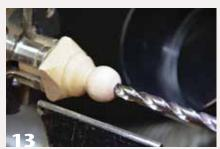
Remount the unturned head blank. Turn most of a sphere, but leave some supporting wood for drilling. First drill a larger hole for the beak, then a smaller hole within the first for reverse-mounting on a screw chuck to finish turning the back of the head.
