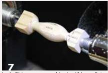
Mark and center punch the ends of the wing blank. This non-square blank will leave flats after turning, so the wings can be cut away safely at the bandsaw.
