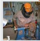
Don wears a helmet and heavy-duty faceshield during initial turning. Turning compromised wood poses extra safety hazards.
