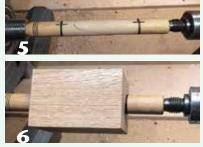
Registration marks on the wedge mandrel help in positioning the turning blank. Advancing the tailstock handwheel applies pressure inside the blank and holds it securely for turning.
