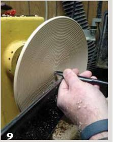
Beading continues in stages on the platter's top, again leaving bulk in the center for support. After completing all the beads, the sharp corners of the small circle left in the center are rounded over with a detail gouge. Burn the valleys on the top of the platter.
