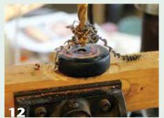
Drill a  $\mbox{\ensuremath{\%}}"$  hole through the baked clay disk, then mount it on the turned mandrel using thick CA glue.
