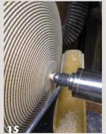
Reverse-mount the platter using a jam fit, and turn away as much of the small tenon as possible. Remove the piece from the lathe, cut away the remainder of the tenon with a flush-cut saw, and sand the small center area on the platter's bottom.
