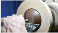
4. The bowl is in and snug, and you are ready to turn the base slightly concave. To remove the bowl from the wasteblock, turn it over and tap the wasteblock on the bed of the lathe.
