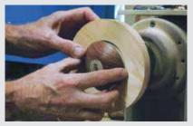
**3.** Turn the lathe off while testing the fit. It must be snug or the bowl will fly off the lathe. If the fit is only slightly loose, a piece of paper towel may take up the slack. A light spray of water may also swell the fibers of the wood, making for a better fit.
