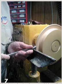
Beading begins on the first stage of the top of the platter, leaving the center thickness for support. After thinning the section to about  $\frac{1}{4}$ , the beads are scored and then cut with the beading tool. The  $\frac{3}{16}$  rim bead is rounded over with a negative rake scraper to blend the top and bottom beads together.
