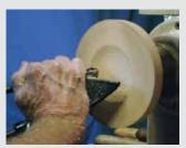
Excavate some of the wasteblock inside your marked diameter to allow space for the island inside the bowl.
