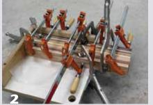
Use plenty of clamps when gluing the strips together. Shown here is the author's clamping jig, which helps keep the pieces from moving during glue-up.
