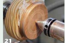
Reverse-mount the platform using a jam chuck. Turn away the wasteblock and form the bottom.
