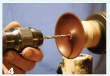
Turn away the inside of the bowl, leaving a raised island in the center. Drill a hole centered in the island that will later accept a tenon turned at the base of the flame.
