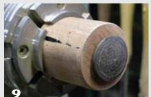
Form a recess in the wasteblock to accept the lid's tenon with a friction fit. Turn the top of the lid. After sanding, drill a small hole in the center to later accept the handle.
