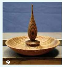
Glue the flame's tenon into the hole in the bowl, and you are ready for finishing.
