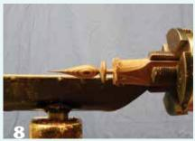
Mount the flame stock in a set of pin jaws and turn a flame shape on which rings can be stored. Turn a tenon at the base of the flame to fit the hole you had drilled inside the bowl section.
