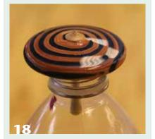
The top of a bottle works well as a holding method for finishing the clay top. Lacquer is not recommended, as it will make the clay sticky.
