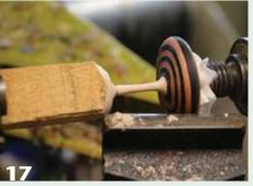
Use tailstock support while turning the top of the disk and wooden stem. Here, a live center is used with its center point removed; a folded paper towel protects the turned surface.
