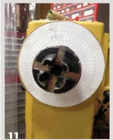
The indexing wheel is mounted over the spindle and held firmly in place with the chuck.
