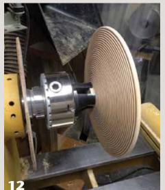
The platter is held by its now small tenon in preparation for indexing both the top and bottom.
