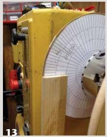
The vertical riser of the indexing board is aligned with one of the lines on the indexing wheel. Now you're ready to draw lines.
