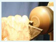
Two methods of reverse-mounting the bowl for turning the base: friction-fit the bowl into a recess in a scrap of softwood (see sidebar) or use a vacuum chuck. In either case, use sharp tools and take light cuts to form a slightly concave base.
