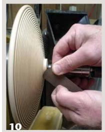
Reverse-mount the platter, reduce the tenon to about 1" diameter, add more beads, and burn lines in the valleys between those beads.
