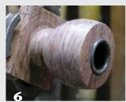
(4-5) Affix and turn the collar material on a wasteblock, forming a rounded ring on the outside and a stepped shoulder on the inside.
