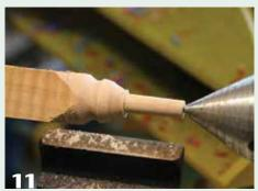
Turn the tailstock end of a wood blank down to 3/8" diameter.
