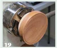
Mount a blank for a spinning platform by gluing it to a wasteblock. Turn the top slightly concave.
