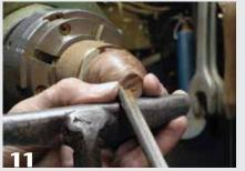
Form a tenon on a wasteblock to accept the vessel's opening with a friction fit. The mounting is reinforced with double-sided tape, but light cuts and steadying fingers are recommended while cleaning up the foot.
