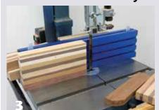
The jointed and planed blank, ready for resawing into board layers.
