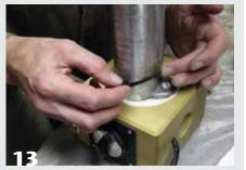
Turn a slender, tapered section for the handle. You can put a slight curve in the wood using a luthier's bending iron, keeping the wood wet during this process.
