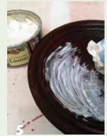
Apply liming wax liberally, then wipe off with a paper towel. The wax will remain in the open pores, accentuating the grain. After wiping off the excess wax with a paper towel, a "foggy" layer will remain but can be removed with 0000-steel wool.
