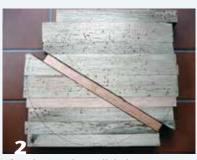
After the initial, parallel glue-up, the blank is cut at an angle and an additional piece glued in.
