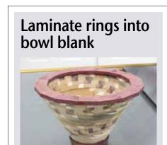
The glued-up stack of rings, plus the base and rim, ready to be remounted on the lathe for the final shaping and sanding.
