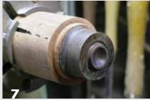
Mount the lid material onto a wasteblock and form the inside of the lid, making a tenon, or stub, that can be used to jam chuck the piece for turning its top.
