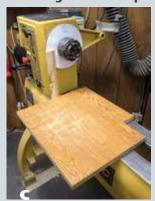
Indexing board in position and anchored to the lathe bed with several rare earth magnets. The top of the vertical riser aligns with the indexing wheel's spokes at the lathe's center height. The pencil jig slides easily on the board's smooth surface.
