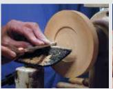
2. A shopmade "friction fit" tool (simply a square nose scraper with a notch ground in the side) helps to cut a square rabbet and allows for gentle cutting inward and to the left for widening the turned recess a little at a time. The bowl should fit snugly into the recess, so it may be necessary to "sneak up" on just the right fit.
