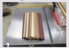
Arrange a selection of various wood strips to make the blank that will become the board you use for the rings.
