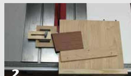
The saw is set up for cutting staves. An adjustable stop block, at left, ensures each stave is cut at identical width. The saw blade is tilted to the required bevel angle, in this case, 13°.
