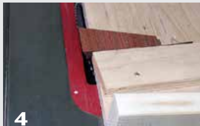
3 The ends of staves must also be beveled so they will sit flat when assembled into a cone. Set the saw blade's bevel to one-half the cone angle—in this case, 30°.
