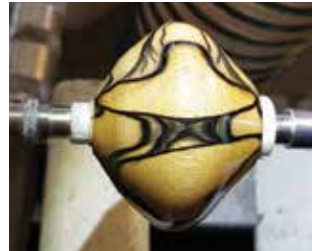
For further refinement, this hollow ornament body was remounted on a pen mandrel with soft duck-call bushings.
