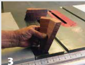
3 The ends of staves must also be beveled so they will sit flat when assembled into a cone. Set the saw blade's bevel to one-half the cone angle—in this case, 30°.
