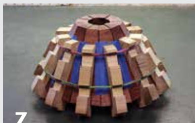
Tape the staves into a fan pattern and dry-fit them prior to gluing. Cauls and rubber bands hold the staves in place.
