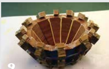
Apply a liberal amount of wood glue and clamp with rubber bands. Two opposing joints are not glued yet, forming two halves of the bowl blank.
