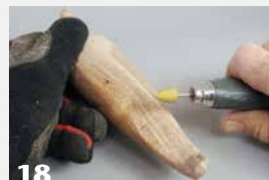
Carving burrs driven by rotary tools help refine and smooth the final pepper shape.
