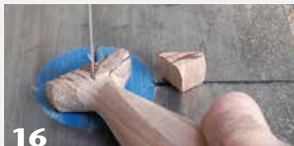
Draw on the ends where you would like to remove material, leaving a stem on one end and a curved tip on the other. Never cut a round object on the bandsaw without proper support; note the flat surface of the workpiece making contact with the bandsaw table.
