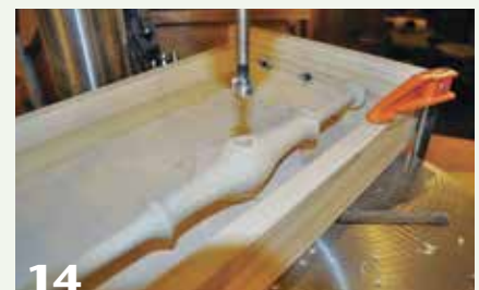
All three legs are held securely in this simple drilling fixture by pressure from bolts at each end. Set the fixture to the correct angle and drill all the leg holes. The one stretcher that receives a mortise is also held in the drilling fixture. Its hole is drilled at 90 degrees, so the fixture is set flat to the drill press table.
