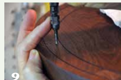
I often decorate the seat top with a defined, textured area. I use a flex-shaft tool with a hammering handpiece to create the texture.
