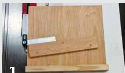
The author's shopmade table saw sled for cutting tapered staves, set for a miter angle of 7.6°. Since the digital protractor is aligned with the left edge of the sled, its angle is set to the complement of the miter angle: 90^\circ - 7.6^\circ = 82.4^\circ .
