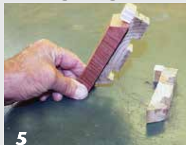
These cauls will make gluing easy. The notches hold rubber bands in place for clamping.
