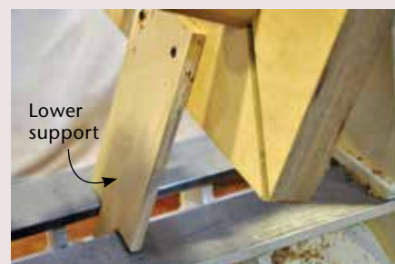
The main platform comprises two layers of \frac{3}{4} "- (19mm-) thick Baltic birch plywood, 16" (41cm) square, glued together. Round adjustable support blocks, 3\frac{1}{2} " (9cm) long and 2" (5cm) in diameter, slide on diagonal slots and are bolted in position with \frac{5}{16} " (8mm) carriage bolts. The lower support, made of \frac{1}{2} "- (13mm-) thick plywood, is cut to fit in and slide along the space between the bed ways to prevent the jig from pivoting during drilling. (The slot in the top section of the platform is used for clamping smaller workpieces.)
