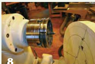
A screw held in large chuck jaws provides ample support for turning the seat.
