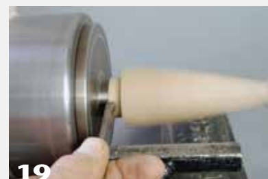
The box is mounted on expanding pin jaws to refine the tight fit of the lid. Use a sharp parting tool to lightly trim the tenon until you reach your desired fit.
