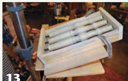
All three legs are held securely in this simple drilling fixture by pressure from bolts at each end. Set the fixture to the correct angle and drill all the leg holes. The one stretcher that receives a mortise is also held in the drilling fixture. Its hole is drilled at 90 degrees, so the fixture is set flat to the drill press table.
