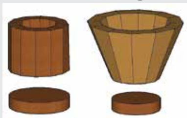
Figure 1. Basic-stave design, left, is straight-sided; tapered-stave design, right, is cone-shaped.
