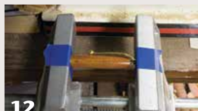
12 The pen kit parts are press-fitted together, with no glue. There are many ways to do this; a vise works nicely, but protect the metal plating on the parts.
