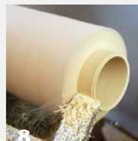
With tailstock support, reduce the diameter of the blank and form a tenon onto which the lid will fit snugly. Fine-tune the fit carefully with a skew held flat on the toolrest.
