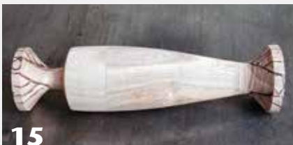
Draw on the ends where you would like to remove material, leaving a stem on one end and a curved tip on the other. Never cut a round object on the bandsaw without proper support; note the flat surface of the workpiece making contact with the bandsaw table.
