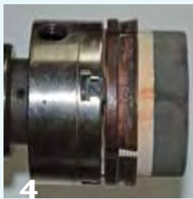
4 Use a rubber pad glued onto a wood block for reverse turning.
