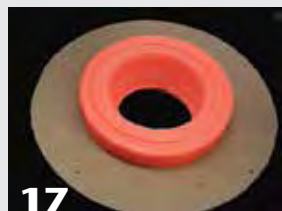
17 The fourth layer. Although the casting is tapered, I easily removed it because of Oogloo's flexibility.
