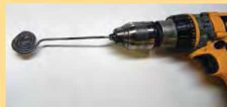
The wire mixer; its end curled into a spiral.
