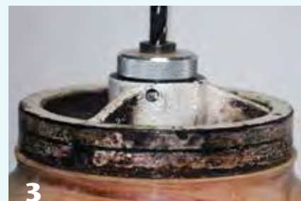
3 Drill the centering hole \frac{3}{8} " deep.
