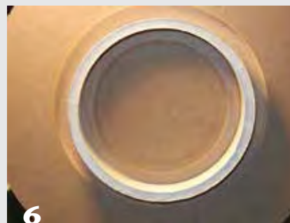
6 Cut two recesses, about \frac{1}{4} " deep. Cut one past the I.D., the other past the O.D. of the groove that holds the coupling. The recesses should each extend past the groove about \frac{1}{2} ". (Coupling installed for clarity.)
