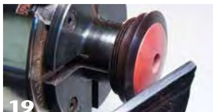
19 Cut a recess in top of the lid, glue a disk of pink ivory, turn it to shape, and drill a shallow hole for the lid's center button.
