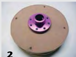
2 Attach a faceplate to the first section, then attach the second section from the headstock (faceplate) side.
