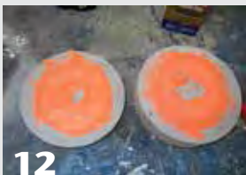
12 Each side of the mold is slightly overfilled with Oogloo. The coupling is then pressed into place (not shown).
