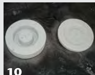
10 I sprayed the completed mold with primer and lacquer, and sanded it for a smooth inner surface.
