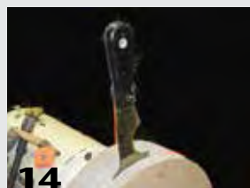
14 After removing the screws, carefully pry the mold apart.
