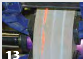
13 The mold is filled, the coupling is installed, and the assembly is screwed and clamped. The excess squeeze-out is easily trimmed once the casting is removed.
