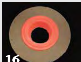
16 The third layer. The protrusion in the casting resulted from inserting the coupling after filling the mold.
