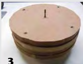
3 A hole drilled in the center of each disc helps align the sections.
