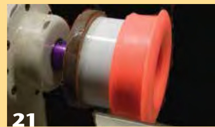
21 Cut a permanent MDF disk and epoxy a new coupling into a groove. This time, cut slightly larger to allow some space for the epoxy.
