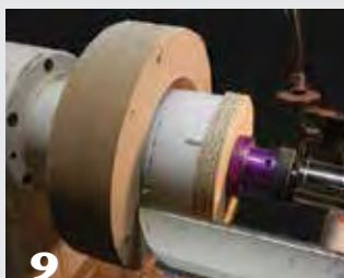
9 This setup shows how to cut the length of the coupling. A reverse-chucking adapter is shown, but a live center will work.
