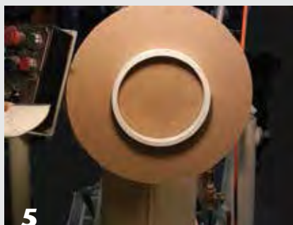
5 The coupling is installed into the second section's groove with a friction fit. (Some couplings have small nubs around their perimeter. These should be carefully sanded away.)
