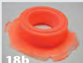
18b The mounting base with the coupling still inside.
