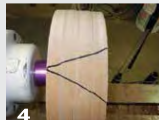
4 Once assembled discs are turned to size, draw several marks on the outside to aid future alignment.
