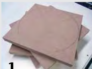
1 Cut five discs from \frac{3}{4} " MDF (fifth disc not shown).
