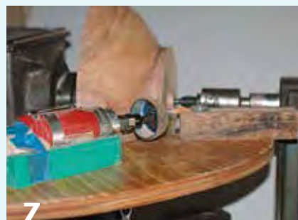
7 Make a table and two sleds, one for an angle grinder and one for a pencil.
