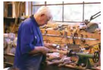
The author is turning one of 97 balusters. The lathe never stops as he measures a critical element.
