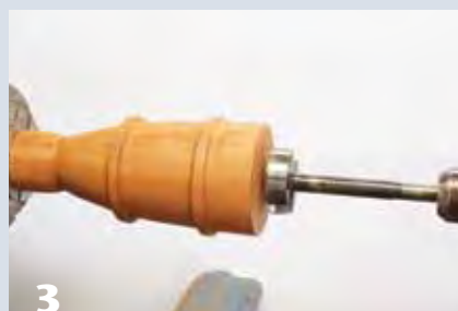
3 Use a saw-tooth drill bit to drill out most of the inside waste.
