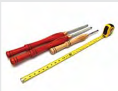
Some of the most popular tools from EWT are the round finisher (Ci0) and square rougher (Ci1), both with 16" (400 mm) handles, and the shorter Ci3m mini-finisher. The Ci stands for "carbide insert."
