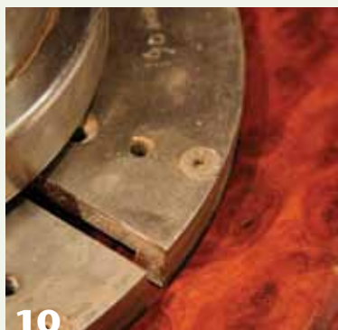
10 You need only a narrow recess for chuck jaws to grip when the recess diameter closely matches the diameter of the chuck's jaws.
