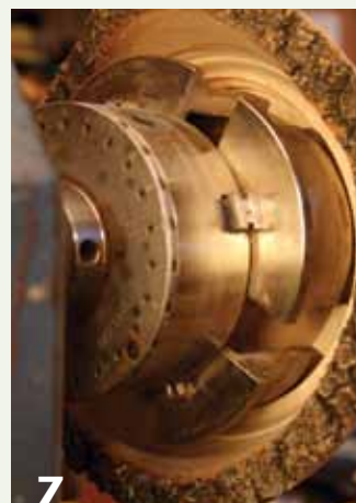
7 Deeper/longer jaws are needed for natural-edged bowls when remounting them to complete the outside profile.
