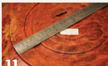
11 This 20"- (505 mm-) diameter jarrah burl platter was held onto the lathe using 8"- (200 mm-) diameter dovetail jaws expanding within a shallow groove. Keeping sufficient mass in the center of this platter gives more margin for error when hollowing.
