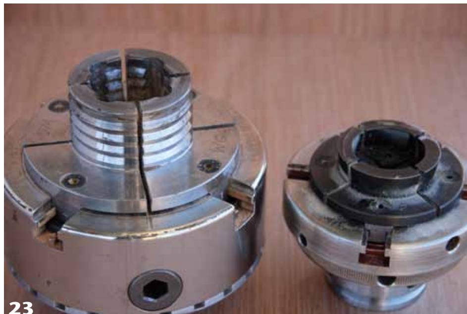
23 Look for dovetail jaws where the inside profiles provide a continuous arc ( right ). Avoid jaws where the inside profile of the jaws is broken ( left ).
