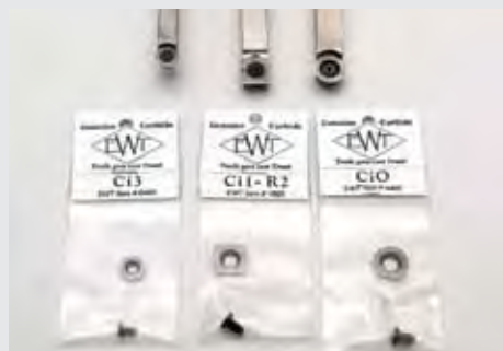
The Ci1-R2 (center) is a new insert for the square rougher that has a very slight curve along each of its four edges. Designed for working smaller bowls, its corners leave fewer scratches.
