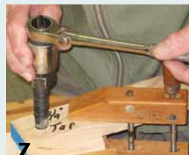
7 Use the first tapped hole to align and tap subsequent holes.
