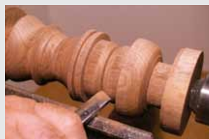
The shaft on the carbide-tipped skew from PSI is oval so it rolls gently on the toolrest which, combined with its very sharp factory edge, makes for easy chamfers, wide V-grooves, and rounded shoulders.
