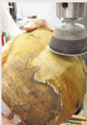
Sanding pin cherry with blue stain, zone lines, bleaching. The glue line on left-hand side of the bowl is cyanoacrylate.
