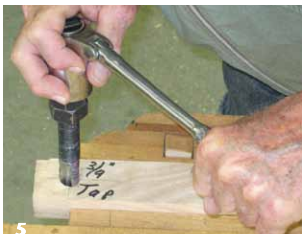
5 Tap the first hole into a scrap piece of hardwood. Make sure the tap is held perpendicular to the wood.
