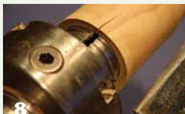
8 Avoid using jaws in expansion mode with endgrain projects. The wood grain is rarely strong enough unless there is sufficient wood around the chuck jaws.
