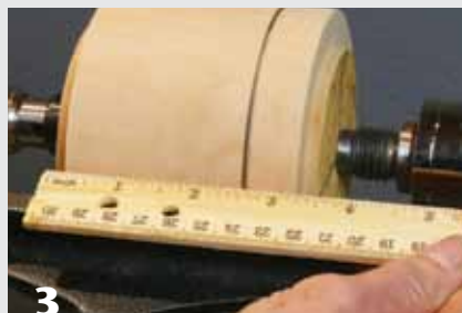
3 Turn a cylinder for the box and lid. Establish a tenon on each end. Mark measurements for top and bottom of the box.
