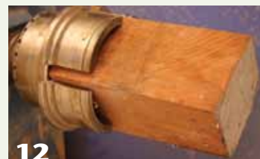
12 Corners of a squared blank should be placed between the jaws of the chuck.
