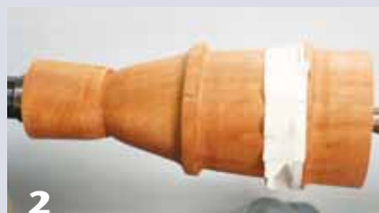
2 Wrap masking tape around the top ring and mark the circumference. Remove the masking tape and mark the tape so that you have three equal parts. The legs will be attached at those three points.
