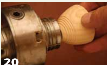
20 The diameter of this small bowl matches the diameter of the chuck jaws when the jaws are almost closed.
