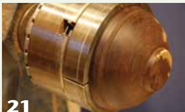
21 The rim of this gidgee bowl fits the chuck exactly. I will turn away the foot and the jaws will not leave a mark on the wood.
