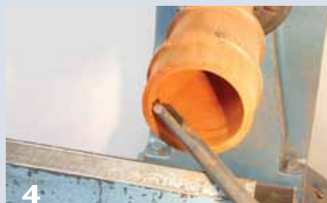
4 Use a bowl gouge with a low-angle grind on the bevel to turn out additional waste.
