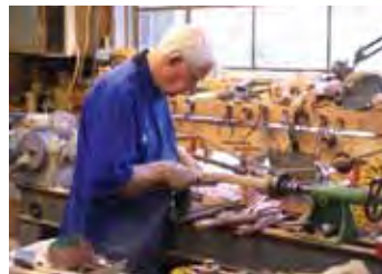
Myron Curtis uses his left hand to act as a steady rest to decrease vibration.
