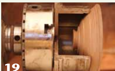
19 Smooth dovetail jaws can grip on next to nothing without marking the wood.
