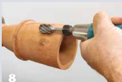
8 A die grinder can quickly remove waste between the points where the legs will be attached.
