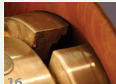
16 Locate expanding jaws on small grooves or beads so that you can finish a base or attend to other details on the outside of a platter.
