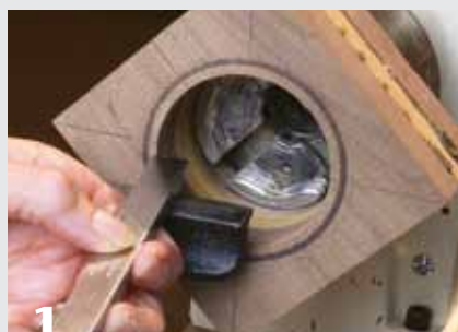
1 After predrilling a hole with a Forstner bit, enlarge the opening of the bracelet to a predetermined diameter. Draw a circle to indicate the finished inside diameter.
