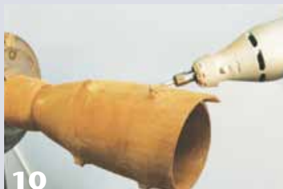
10 A rotary tool with a small round-end burr is ideal for cleaning up around the raised points.
