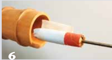
6 A shopmade cylindrical drum sander works well to sand the inside.
