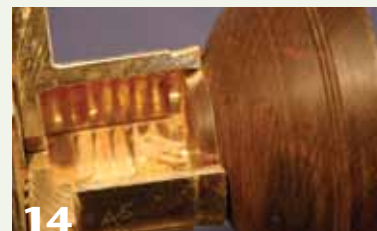
14 Long jaws with smooth rims can grip on details of a profile without damaging the wood when the diameters of the bowl and jaws match.
