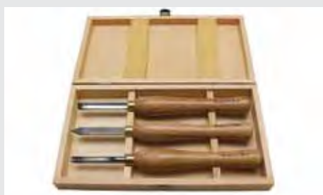
PSI's boxed set of three lathe tools (gouge, parting tool, and skew chisel) with brazed-on carbide tips are 11" (280 mm) long overall and are ideal for the casual turner who does not want to invest time in a sharpening regimen.
