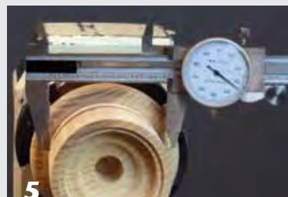
5 Transfer the measurement from the inside diameter of the bracelet to the outside diameter of the box so that the bracelet will slide easily over the outside of the box.
