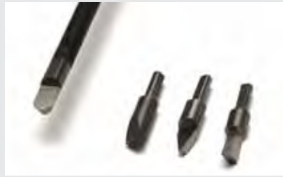
The New Edge pen tool has four carbide tip profiles: round nose, skew, diamond and parting tool. All tips work beautifully on spindles and bowls, too. The tips are changed with an Allen screw.
