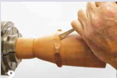
9 Using a fishtail gouge to remove waste between the raised sections is a peaceful way to work.
