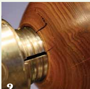
9 A faceplate-turned bowl is subject to cracking when expansion chucking.
