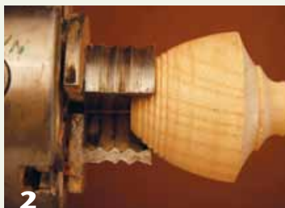
Simple dovetail jaws can grip on next to nothing.
