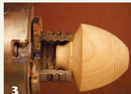
The detail on the shoulder of this small vase provides a groove on which the dovetail jaws grip.
