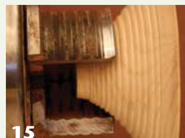
15 The beads on the outside profile of this small vessel provide grooves for long dovetail jaws to grip.
