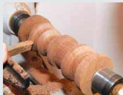
The Ci0 Easy Finisher has a round carbide cutter that is perfect for doing inside work on smaller bowls, and for creating large coves on spindle work. Here it is shown working kiln-dried walnut.
