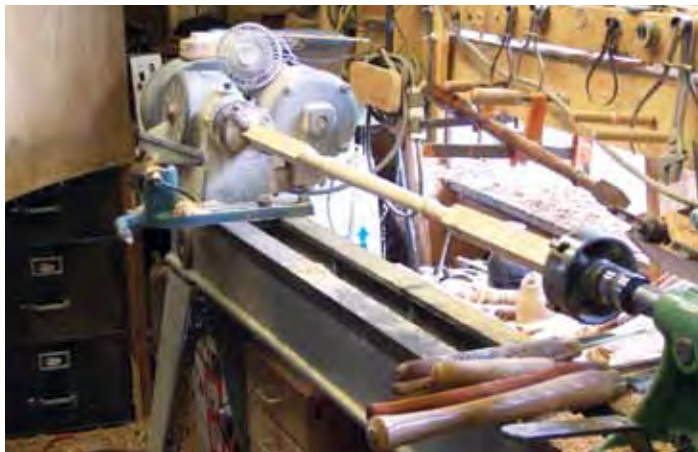
Two, four-jaw chucks—one mounted on the headstock, the other mounted on the tailstock—aid in dampening vibration when turning long, thin spindles.
