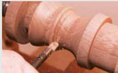
The round-nosed insert for New Edge's pen-turning tool is ideal for creating small coves on the rims of bowls, or decorative elements on spindles. Carbide-insert cuts are so precise they rarely need sanding.
