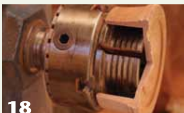
18 If your chuck has serrated jaws that might damage the wood, there are times when you can use the jaw shoulders for holding a project.
