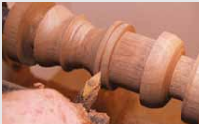
The full-sized diamond cutter from New Edge has a very slightly rounded tip that can be plunged into the work to locate or define a groove. With sharp sides, it replaces a traditional parting tool.
