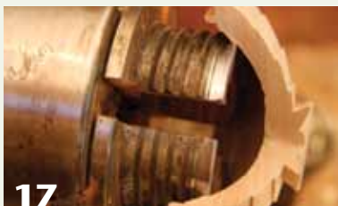
17 This box lid has been cut away to illustrate how a groove on the inside of a bowl can provide a shoulder for locating the jaws. In this case, the chuck is used in expansion mode.
