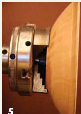
5 These simple dovetail jaws are able to grip as little as a \frac{1}{16} " (1.6 mm) foot or tenon.
