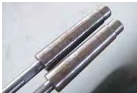
The extent of the problem with tools rusting when near the ocean becomes clear when you unwrap two pen mandrels on a Monday and find the Morse tapers have rusted this much by Wednesday.
