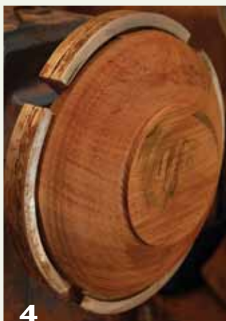
4 When gripping diameters larger than the original inside diameter of the jaws, the corners of the jaws dig into the wood and leave a mark; however, those marks are not a problem when roughing the profile of a thin plate.
