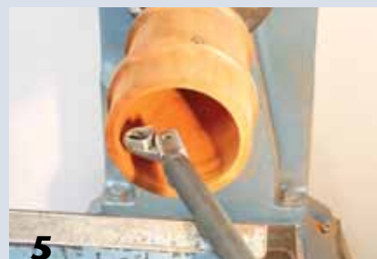
5 A Rolly Munro hollowing tool works well to trim up the waste at the bottom of the vessel.
