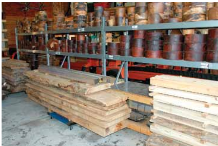
The day's slabs are stickered and stacked in front of shelves full of turning blanks. From here, slabs destined for turning blanks will be cut to specifications using a bandsaw, and the edges waxed to control the drying process.
