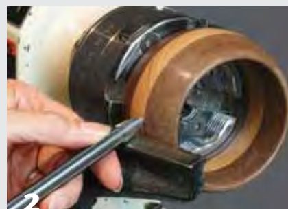
2 Fine-tune the outside curve of the bracelet. Also, shape the edge of the bracelet so that it is flat. Doing so will allow it to fit squarely on the box.
