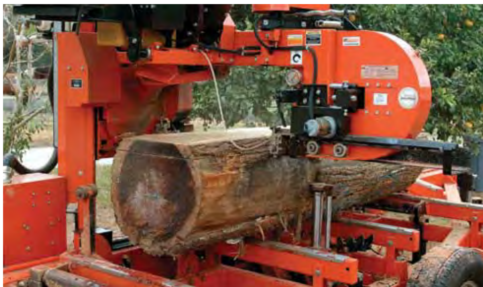
A rainbow poplar log is being cut into boards on a Wood-Mizer. The kerf of the blade is very thin—about \frac{1}{8} " (3 mm)—contributing to the efficiency of the cutting operation and maximum use of the timber.
