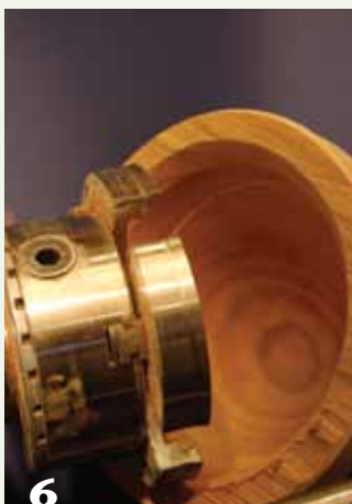
6 Remounting rough-turned bowls for completion of the profile is simplified when a shoulder is turned on the inside of the bowl after the wood had seasoned and distorted.
