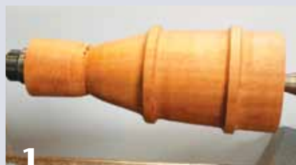
1 Turn the form to shape and leave two raised rings.
