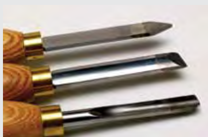
Penn State Industries (PSI) says its carbide-tipped tools may never need sharpening. For short-handled tools, they were a pleasant surprise because they hold an edge so well there is little chatter or resistance.
