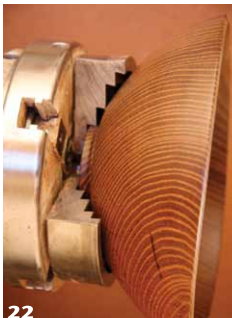
22 Not every bowl will fit into step jaws like this bowl does, especially wide bowls with small feet. Using step jaws, however, often enforces more pleasing proportions on bowls than their maker may have intended.
