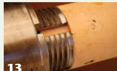
13 A shoulder or bottom of a curve (also see Photo 14 ) seated against the rim of the jaws provides the best grip.
