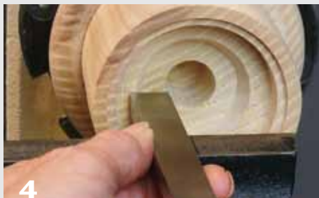
4 Hollow the inside of the box. (You are turning endgrain to make this box, so employ endgrain-turning techniques.)
