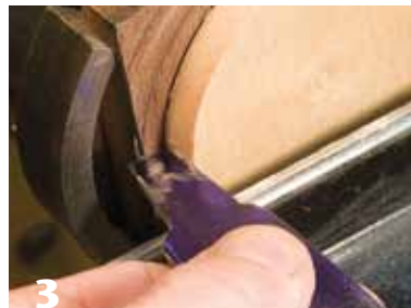
Use the right side of the scraper to cut the outside angle of the plug to match the hole cut in the body of the turned object. Hold the tool at 90° on the toolrest.
