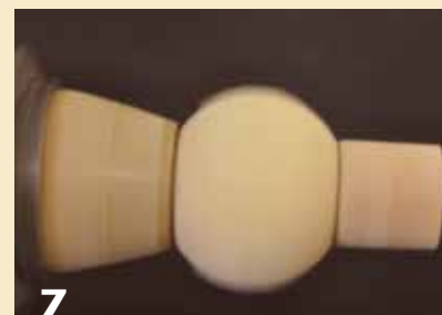
7 With the lathe's speed set at about 1,000 rpm and the ball held in between the cup centers, the revolving out-of-round form creates a ghost around its outer edge. Turn away this ghost.
