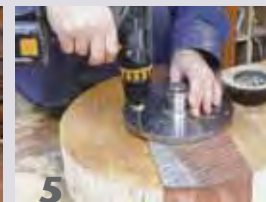
5 Attach an 8" (20 cm) faceplate to what will become the top surface of the final piece. Make sure the faceplate is positioned in the center of the good wood. The large-diameter faceplate allows the screws to be placed in the scrap wood.
