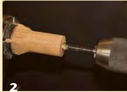
2 Drill a hole in the tailstock cup center. Use a Forstner bit, mounted in a Jacobs chuck.
