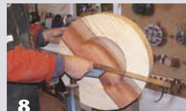
A flat base is needed for the bottom of the wings of the final piece, so check the outside surface with a straightedge.
