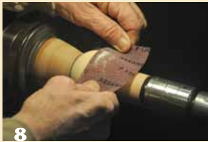
8 Sand the sphere. An Abranet abrasive is used here. Note that the sawdust flows through the mesh of the fabric.
