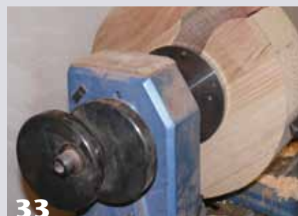
33 Because of the difference between the weight of the good wood and scrap wood, the disc may be unbalanced. My Vicmark lathe has a counterbalance that helps overcome the problem of unbalanced wood.
