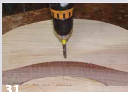
31 Drill a hole for a screw chuck for mounting the disc onto the lathe.
