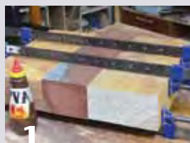
1 The initial glue up consists of two sides of scrap wood with the good wood glued in between.
