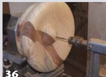
36 Finish shaping the front surface and then sand that area. Drill a hole in the center to take the screw chuck so that the piece can be reversed.
