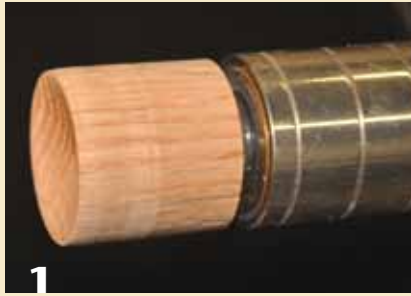
1 The tailstock cup center will ultimately be attached to the live center in the tailstock.
