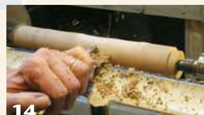
14 Reduce the diameter of the rest of the tube's body.
