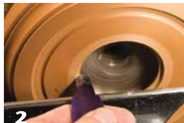
Use the left side of the scraper, holding it at 90° on the toolrest, to finish cut the hole for the plug.
