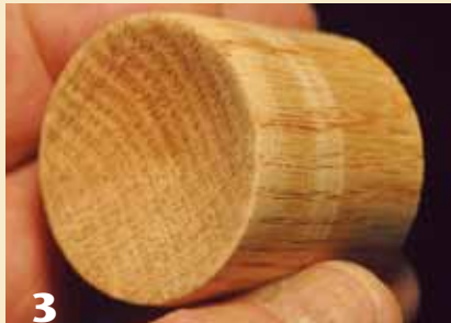
3 The tailstock-end cup center is ready for use. Not shown is the hole drilled in the other end.
