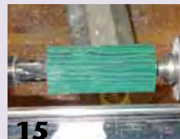
15 Mount the drilled blank between centers of the lathe and turn the handle to shape.
