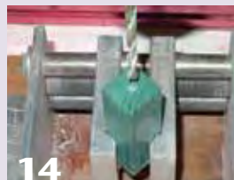
14 For a handle without a pen tube, drill through the blank using a #18 drill bit.
