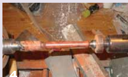
4 Remount the cylinder, finish turn the shape, and apply several coats of CA glue for a durable finish.
