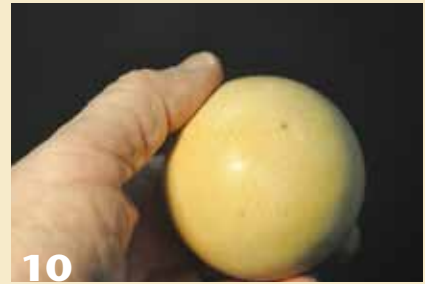
10 A sphere turned, sanded, and buffed in about ten minutes.
