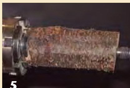
5 Mount a length of freshly cut wood into a four-jaw chuck. Turn it into a cylinder.
