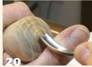
20 Remove the nub using a carving gouge, then sand.
