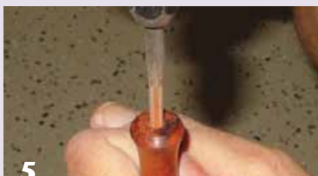
5 Tap the hole using a 5 mm \times 0.80 tap.
