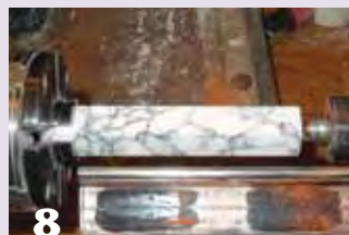
8 Mount the blank into the four-jaw chuck. Use the tailstock for support.
