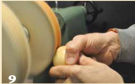
9 When buffing the sphere, hold it tight against the wheel and support it against the direction of rotation.
