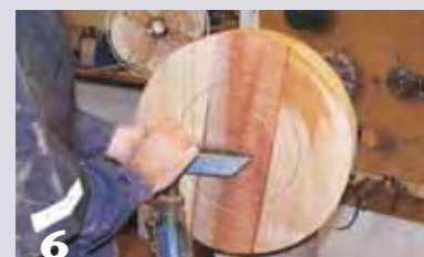
Draw a circle to indicate the diameter of the curved void in the underside of the turning.
