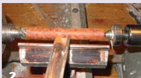
2 Mount the blank between centers of the lathe and turn to a cylinder.
