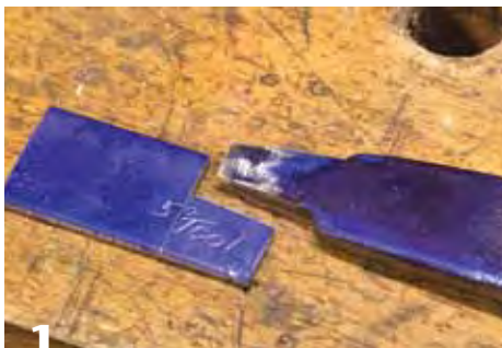
Use a jig to aid in creating a 5°-angled scraping tool, which will be used for cutting matching holes and plugs or matching grooves and inlay rings.
