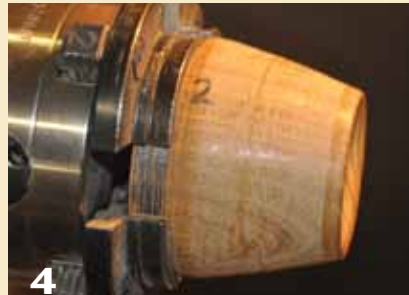
4 Mark the position of the jaws on the headstock cup center so that it can be placed back into the chuck in exactly the same position as when it was made.
