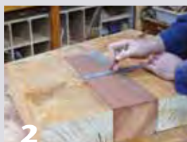
2 Carefully measure the good wood to find its center.
