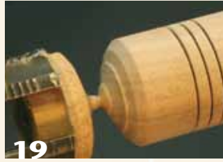
19 Leave a nub of wood attached to the bottom and use a handsaw to part the cylinder off.
