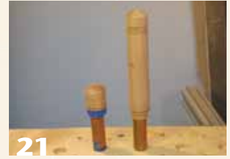
21 A drying board with holes to receive dowels makes spray finishing easy. This system also works great for other small projects.
