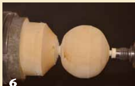
6 Turn the ball into a rough shape, then part it off the lathe.
