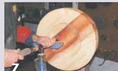
Hollow out the curved void of the underside of the piece. Sand when finished with this section.
