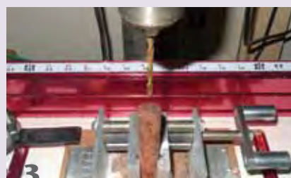
3 Drill a hole that will accept the rod from the razor head using a #19 drill bit. Drill the hole approximately 25 mm deep.
