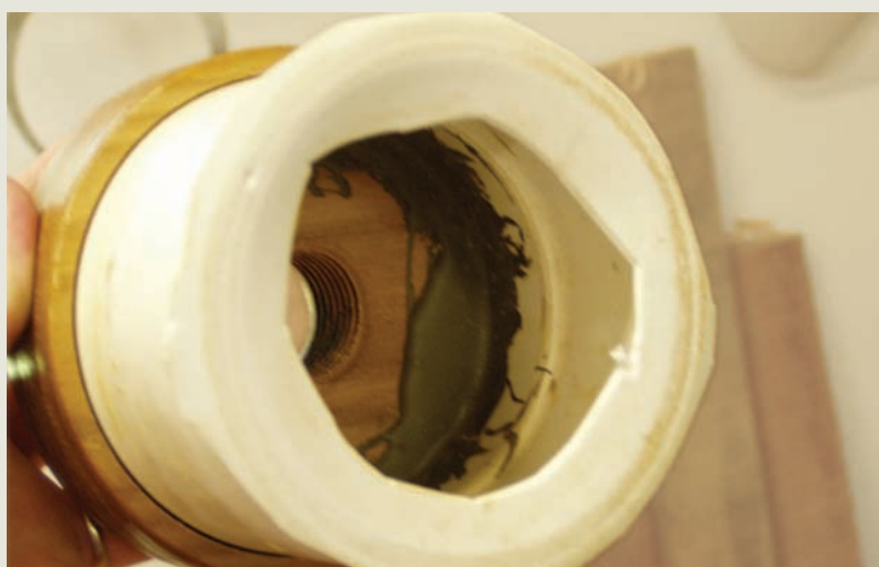
Top view of completed vacuum chuck with gasket in place.
