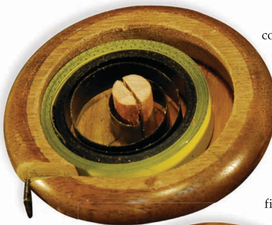
Tape and spring installed, ready to glue the second side to the case.
