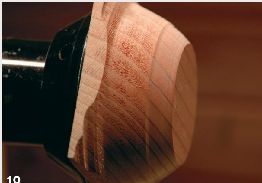
10 Even with an unmagnified view, huge differences are observable in surface finishes. The upper half was cut with a freshly ground M2 bowl gouge, while the lower half was cut with a 2060 bowl gouge, bevel and flute honed.
