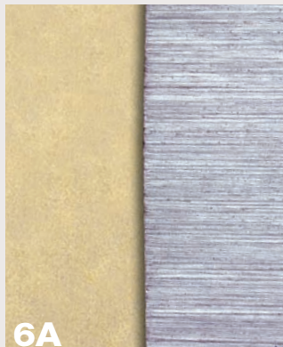
6A Skew chisel edge, bevel ground only (20X).
