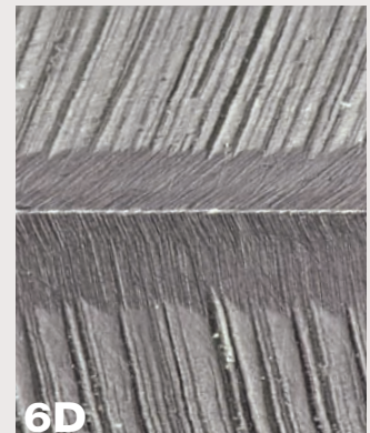
6D Edge view of skew chisel, ground and honed (200X).
