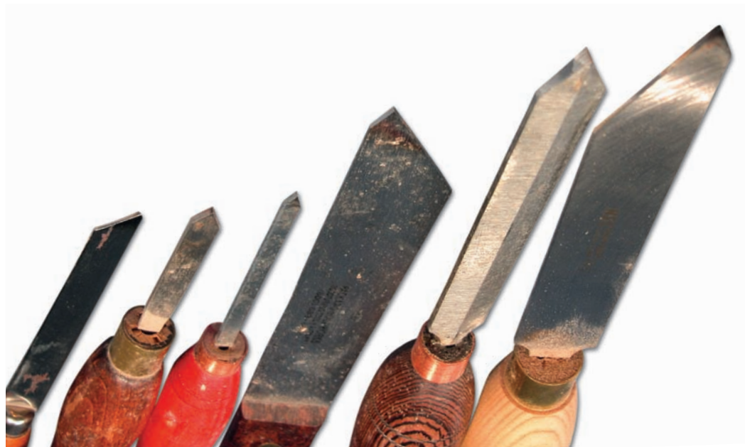
Shown here is an assortment of the author's parting tools. (Left to right) Nick Cook tool with a flute (Sorby), standard diamond parting tool (Sorby), standard thin-walled tool (no flute), shopmade mini tool, Bonnie Klein mini parting tool, and shopmade parting tool.
