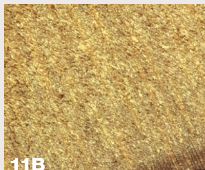
11B Magnification 100X, wood surfaces cut with PM 2060 gouge.
