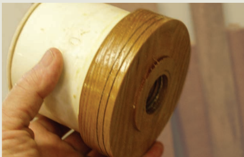
Bottom view of completed vacuum chuck.
