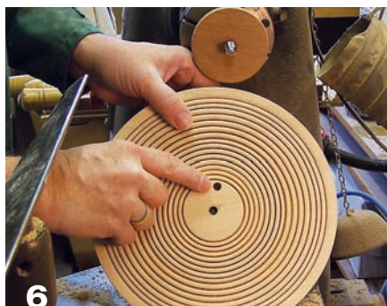
6 Position the new center hole about 1" from the original center.
