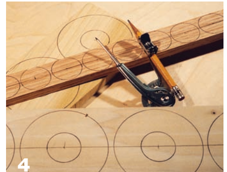
4 To streamline your glue-ups, lay out your tenons directly on the coaster stock.
