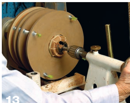
13 With a Forstner bit, true up the inside of the bottom of the vessel.
