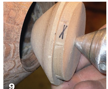
9 Install a temporary bowl base with a tenon.
