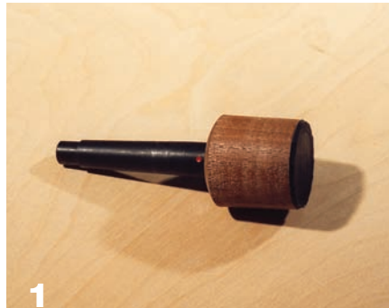
1 Assemble a shopmade friction block mounted on a Morse taper spur drive.
