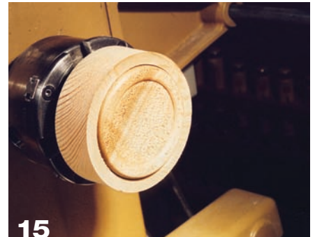
15 After turning away the tenon, sand and seal the bottom.
