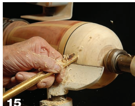
15 A solid piece of 8/4 material (hollowed beforehand) dresses up the vessel's look.
