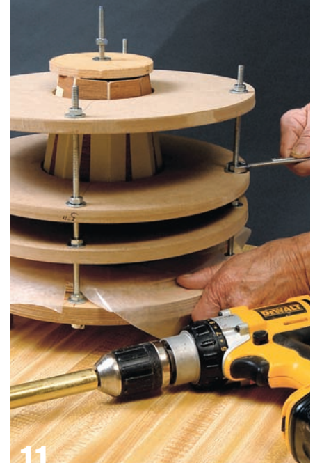
11 After adding three rings, adjust the assembly for even tension. You can also make this adjustment at the lathe.
