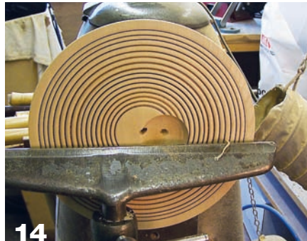
14 Although it looks odd, the hole on the right is the new center of the platter.
