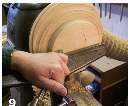
9 Cut away the first recess and make a flat bottom. Then mark for the new recess that will be centered on the new axis.
