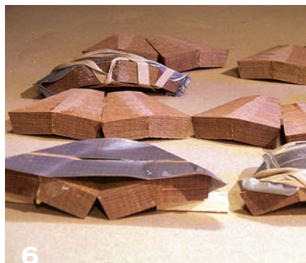
6 Use duct tape as a clamp.
