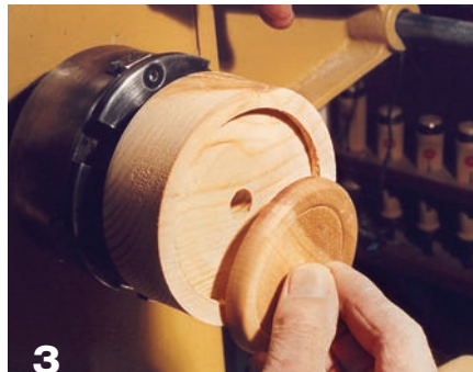
3 A \frac{1}{2} " access hole drilled in your jam chuck will help you remove tight-fitting coasters.
