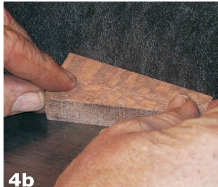
4b Lightly sanding the stave sides will improve the appearance of the glue joints.
