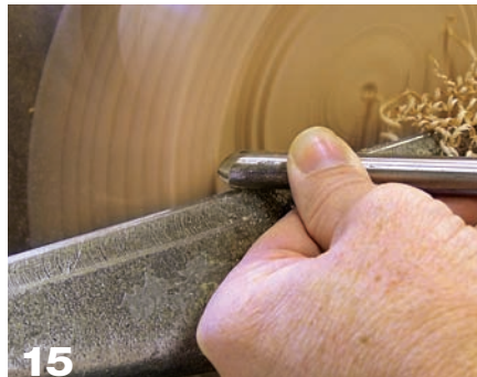
15 To begin hollowing, hold the flute at 3 o'clock. The bevel will head straight into the spinning beads. Once safely past this point, rotate the tool to a more open position.
