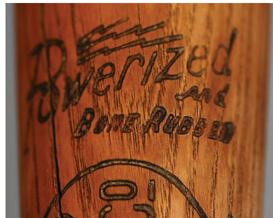
This bat from the mid-1930s shows two Louisville Slugger processes: "Powerized" and bone-rubbed. Rubbing a bone on the bat while it was still on the lathe for even a minute or two would take the place of a player doing this by hand for many hours.
