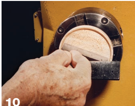
10 Use a straightedge to test the rim for flatness.
