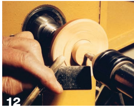
12 Form the bottom using a friction drive supported by a live center.
