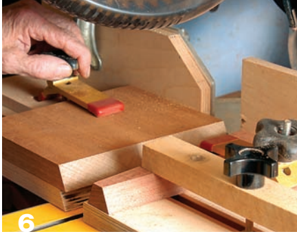
6 To improve the accuracy of your staves, securely clamp a stopblock to your jig.
