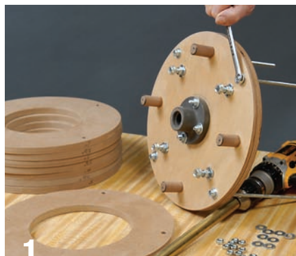
1 With a lock nut and washer, secure four 9" lengths of all-thread rod to the base.
