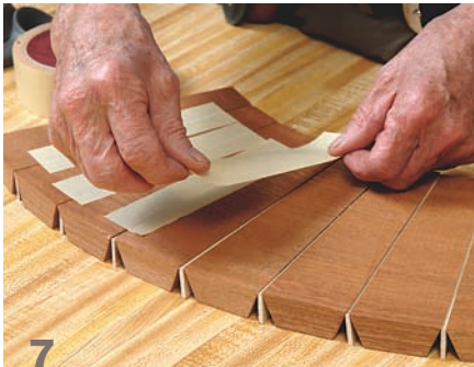
7 Before applying glue, tape together the exterior faces of your staves.
