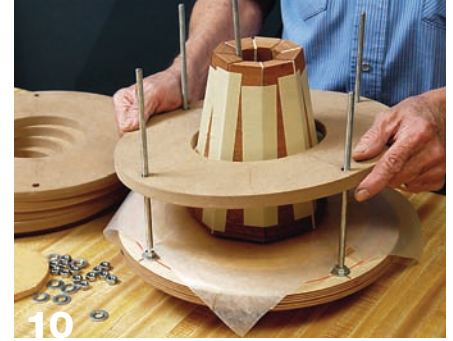
10 Push the first MDF ring to the bottom of the staved vessel, then add washers and nuts.
