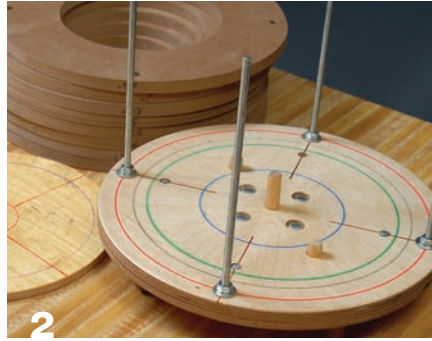
Dowels on the top side of the base help position the floating base.
