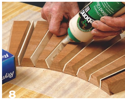
8 Be sure to apply woodworker's glue to one surface of each joint.
