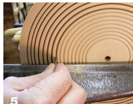
5 Create well-defined details by pushing a thin wedge of dark wood into the spinning grooves. This works most dramatically on lighter-colored woods but can be a subtle accent with darker woods, too.
