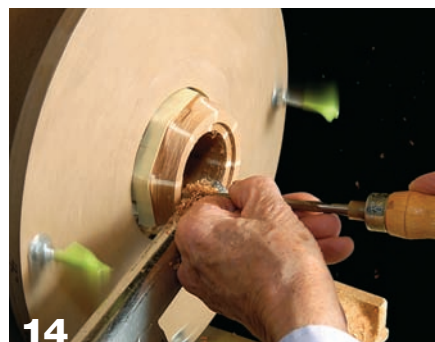
14 Square up the bottom of the vessel, then cut a dado for the bottom piece.
