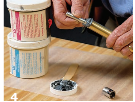
To make a nut driver, epoxy a ¾" nut into a ½"-diameter brass tube.
