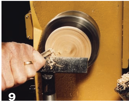
9 Ride the bevel as you cut with your gouge toward the center.
