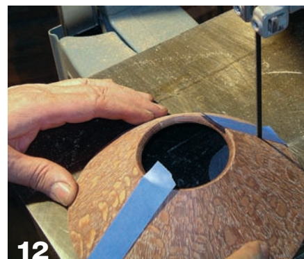
12 Splitting the bowls requires a steady hand. Because the glue line can be difficult to see, the blue tape provides a visual aid.
