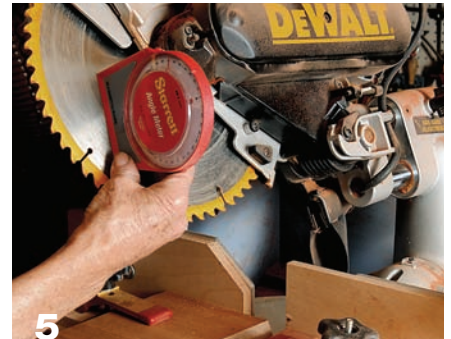
With an angle meter, set the compound mitersaw to 22.5 degrees.
