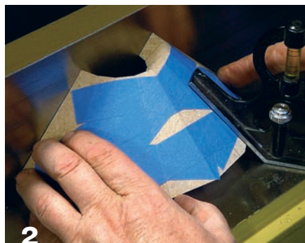
2 At a jointer, check 90- and 45-degree angles.
