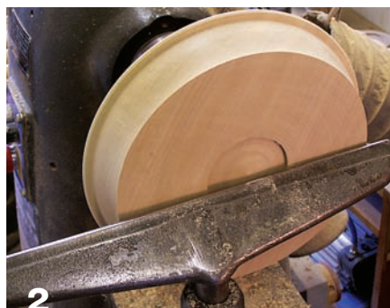
2 Flatten the bottom, make a recess for the chuck, and establish a rounded edge.
