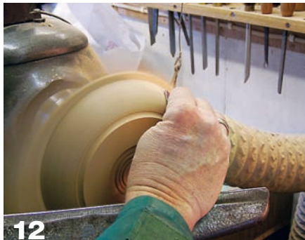
12 Sand what you can on the bottom now, as you won't be able to come back to it later. Sand the overhanging flange of the rim with the lathe off.
