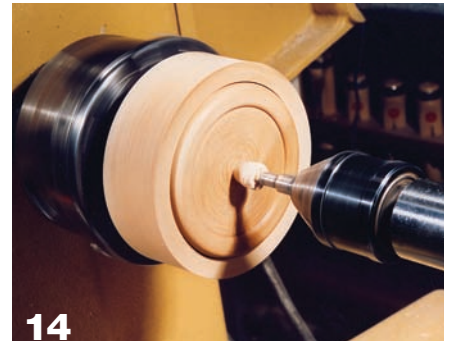
14 With a narrow parting tool or skew, remove the remaining tenon.
