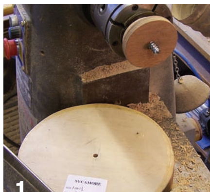
1 Start with a sound blank, roughly 10" in diameter and 1\frac{1}{2} " to 2" thick. Mount the stock on a screw chuck like normal.
