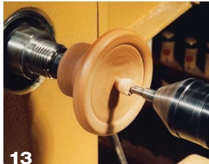
13 After forming most of the coaster bottom, turn down the tenon to a cone.
