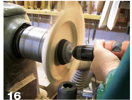
16 With a 3"-diameter soft disc, sand the interior of the bowl.
