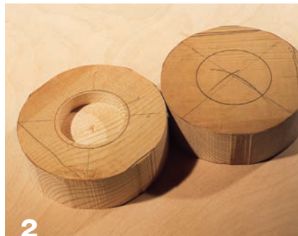
2 Bore your softwood blocks to provide a grip for the chuck jaws.
