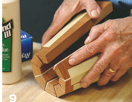
9 Roll up the staves into a circle and fasten with masking tape.
