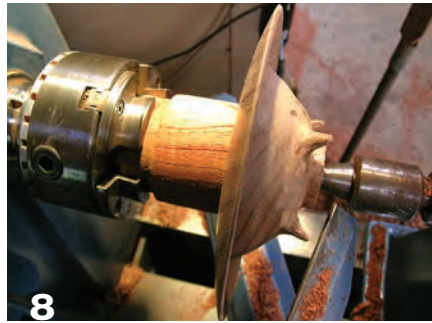
8 Hold the bowl against a mandrel to turn down the temporary chuck spigot.
