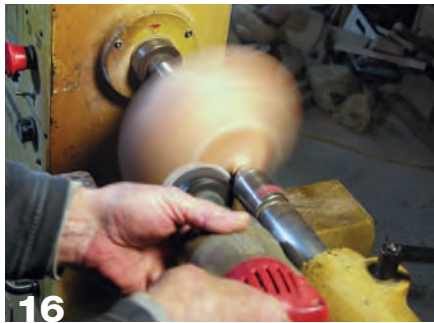
16 Sanding can be done around the stem with a power sander. Just don't let the sander "bounce." You can also sand without the lathe, using the tenon to clamp to a bench.
