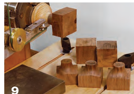
9 Turn down the shoulder of each knob. A belt-driven cutting frame, left, does the work.
