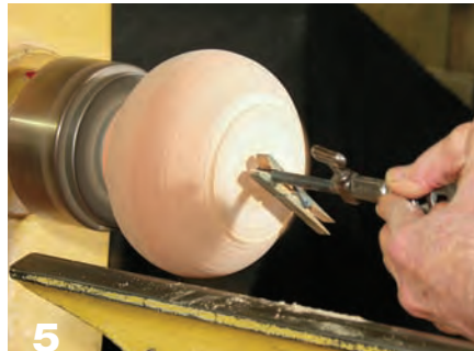
5 Begin hollowing by drilling a 5/16" hole in the bottom of the squashed sphere. The hole should extend ½" from the top.
