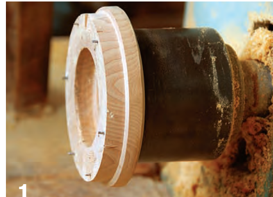
A Japanese jam chuck fits into the metal cup-chuck. Note the protruding nails, which secure the bowl.
