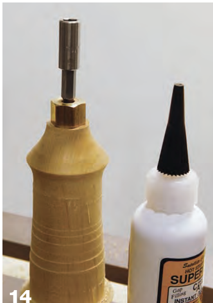
14 Insert the tool-holder shank and adhere with CA glue.
