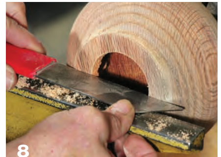
8 The bottom, which will receive the plug, should be faced off so it is flat. A parting tool with a straight shaft makes a handy straightedge.
