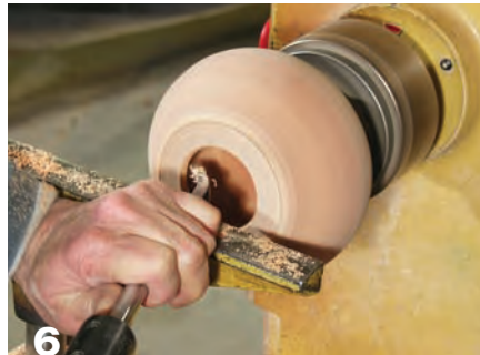
6 Because this is the bottom, you can open a hole as big as you need (within reason). The diameter shown above is 1½".
