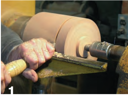
1 Start with a cylinder about 5" in diameter and 5" long and with a tenon turned on both ends for your scroll chuck.
