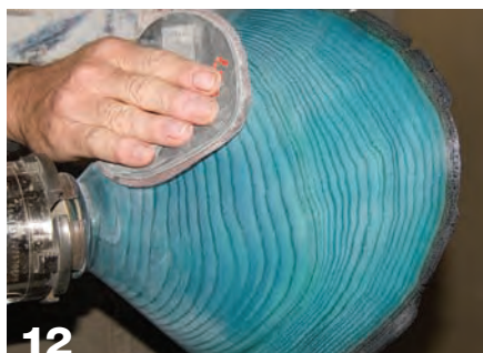
12 Sand built-up coats with a 400-grit disc.
