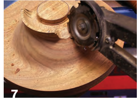
7 For quick removal of stock, use an Arbortech Mini Carver or similar tool.
