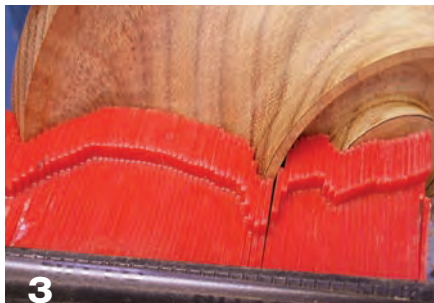
3 Use a profile gauge to check the shape around the legs.
