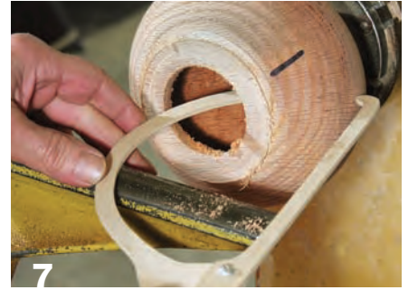
7 Aim for a wall thickness of ¼" or less. As you work around the widest part toward the top of the pod, the thickness should graduate to ½".
