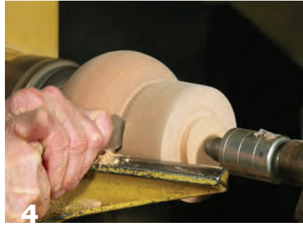
4 Part off the plug material with a parting tool. Use a thin-kerf parting tool, which will help match grain later (less stock removed).
