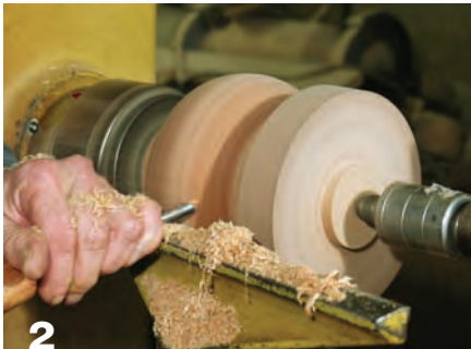
2 Begin shaping the pod form. As you shape it, you can reduce the diameter of the plug material.
