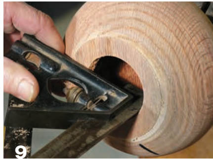
The inside wall to which the plug is fitted should be square to the bottom. Use a combination square, as shown above, to check your fit.
