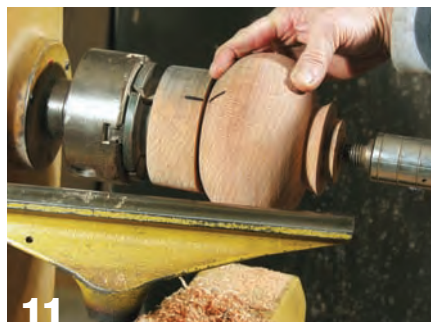
When the plug fits snugly, apply medium CA on the plug and flange of both the plug and the pod. Align the marks and bring up the tailstock for pressure.
