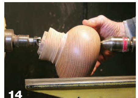
Replace the hollow tailstock center with a cone live center and take up normal pressure on the tailstock. Make sure each driver spur has a good bite in the wood.
