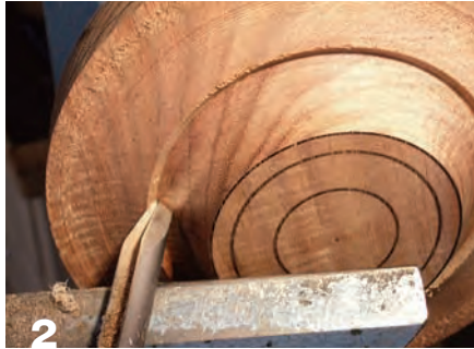
2 Mark the outside of the bowl and foot before you begin turning.
