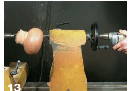
Using a spurred drive center, set in the original center of the plug material with two spurs in the wood. Turn the pod to the place where you want the opening to be.
