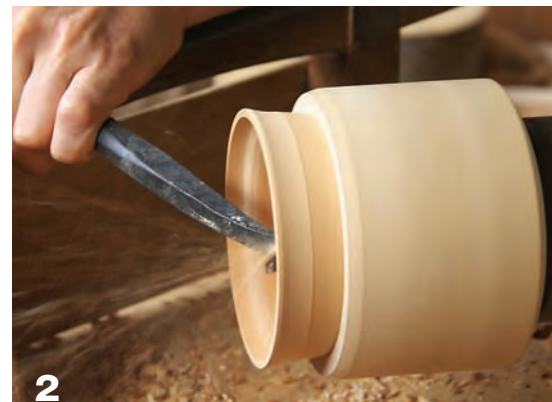
A wooden jam chuck holds the bowl while the turner shapes the inside with a hook tool. Rotation is clockwise; the tool contacts the far side of the piece.
