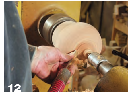
While the glue sets, turn off the tenon and shape the top, leaving enough wood to keep pressure on the plug. Reduce the plug and sand the pod to finish smoothness.
