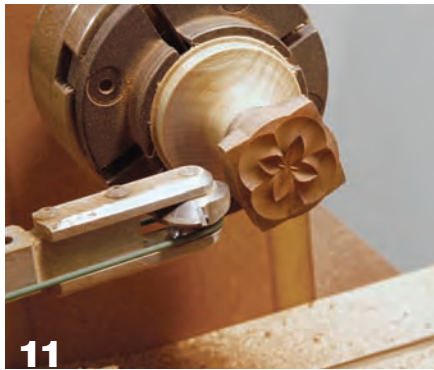
Make the decorative cuts on the face of the knob. Notice how phasing was added to position the points of one pattern in the rounded lobes of another.
