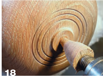
18 Using a freshly sharpened thin-kerf parting tool, cut grooves in the bottom. One of the grooves should be on the glue line, causing it to disappear.
