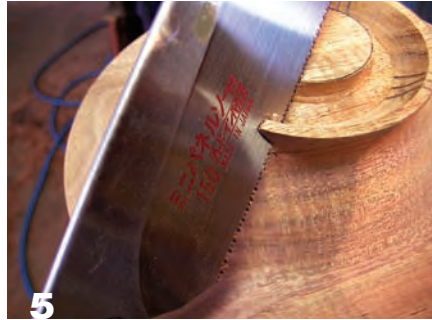
5 Use a pull saw to cut both sides of the legs.
