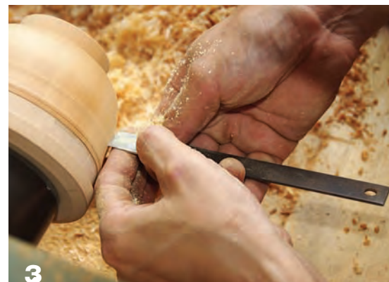
To smooth the surface, the Japanese turners use a kogatana , which is profiled similarly to a cabinet scraper.
