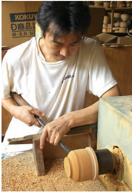
A Yamanaka woodturner profiles the exterior of a bowl on the jam chuck. Note the tool rest positioned on the workstation.
