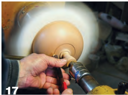
17 To finish off the bottom, make a cup-shaped jam chuck and bring the tailstock into the original center. Reduce the tenon, shape the remaining bottom, and sand.
