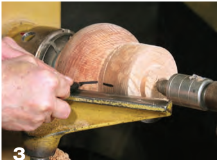
3 With the pod shaped, cut the plug material to a convenient diameter and make a mark from the pod onto the plug material.
