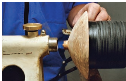
With the tenon and tailcenter as guides, align the bowl on the vacuum cylinder.
