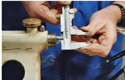
With a vernier caliper, determine the interior diameter of the tailcenter.
