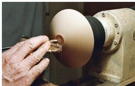
Clean up the bottom of the bowl with a \frac{3}{8} " spindle gouge.
