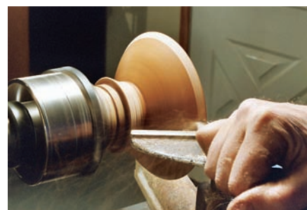
Shape the exterior of the bowl with a small bowl gouge.
