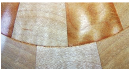
Poor inter-ring flattening or sanding before gluing rings together
