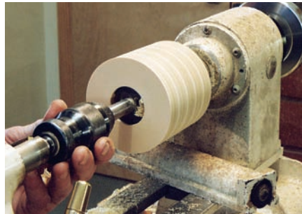
With a 1" Forstner bit, drill a \frac{3}{4} "-deep hole for the 1"×8 tpi nut.
