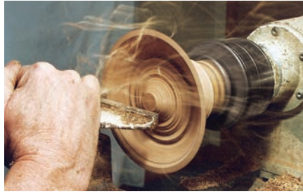
Turn the interior of the bowl. Be sure to leave some mass in the bowl center to help control chatter.
