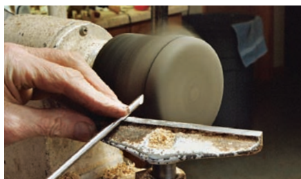
Use the long point of a skew to clean up the exterior of the gasket.
