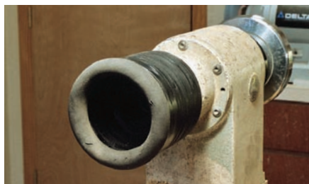
To prevent the gasket from unraveling, wrap the material with electrical tape.
