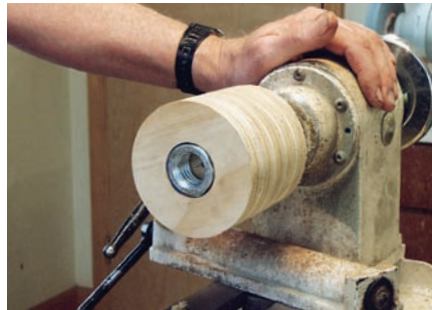
Check to see how the nut fits. Grind off the corners of the nut to help the fit and to allow the 5-minute epoxy to adhere better.
