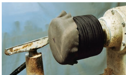
Fit gasket material over 1½–2" of wall.
