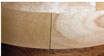
Error in cutting the segment angle accurately
