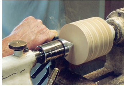
With the small faceplate, turn the stack of plywood blocks to a 3\frac{3}{4} " diameter. A revolving live center in the tailstock will help steady the block.
