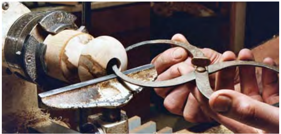
A bent-angle tool is essential in removing stock from inside the globe.
