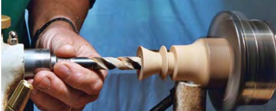
To speed up hollowing of the funnel, remove stock with a \frac{1}{2} " drill bit.
