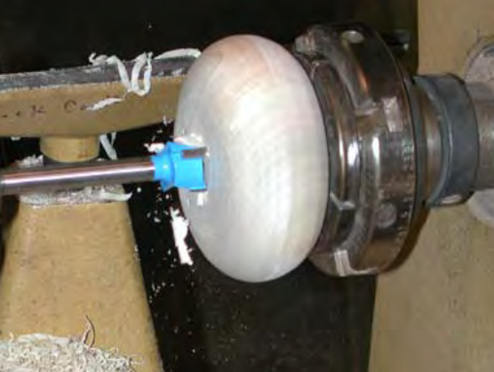
A 0.995" Forstner bit bores a hole perfectly sized for a standard U.S. quarter.
