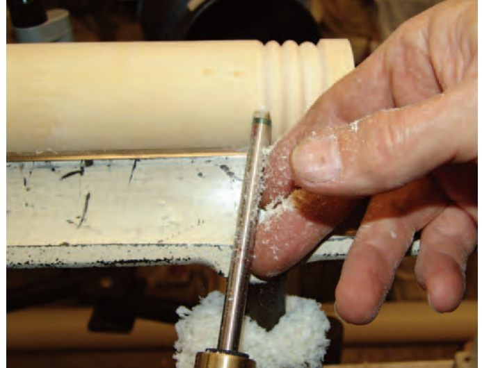
Bead step 2: Drop the handle slightly as you roll the bead "uphill." See further details at left .
