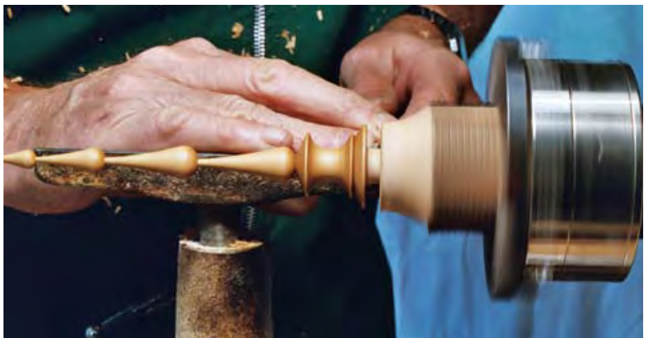
Switch to a small parting tool to turn the tenon that will fit into the globe.
