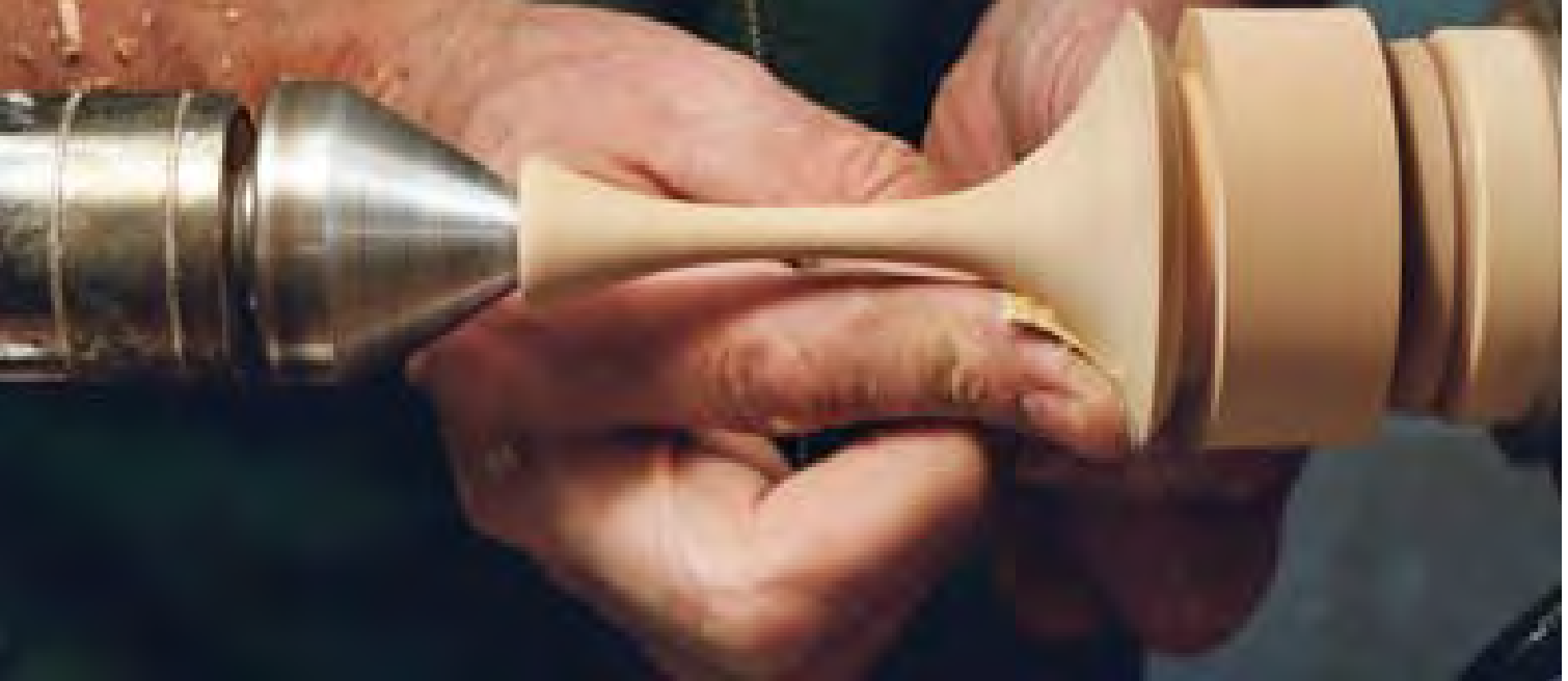
After turning the stem (still supported by the tailcenter), sand the piece smooth with progressive grits of 150-, 180-, and 220-grit papers.
