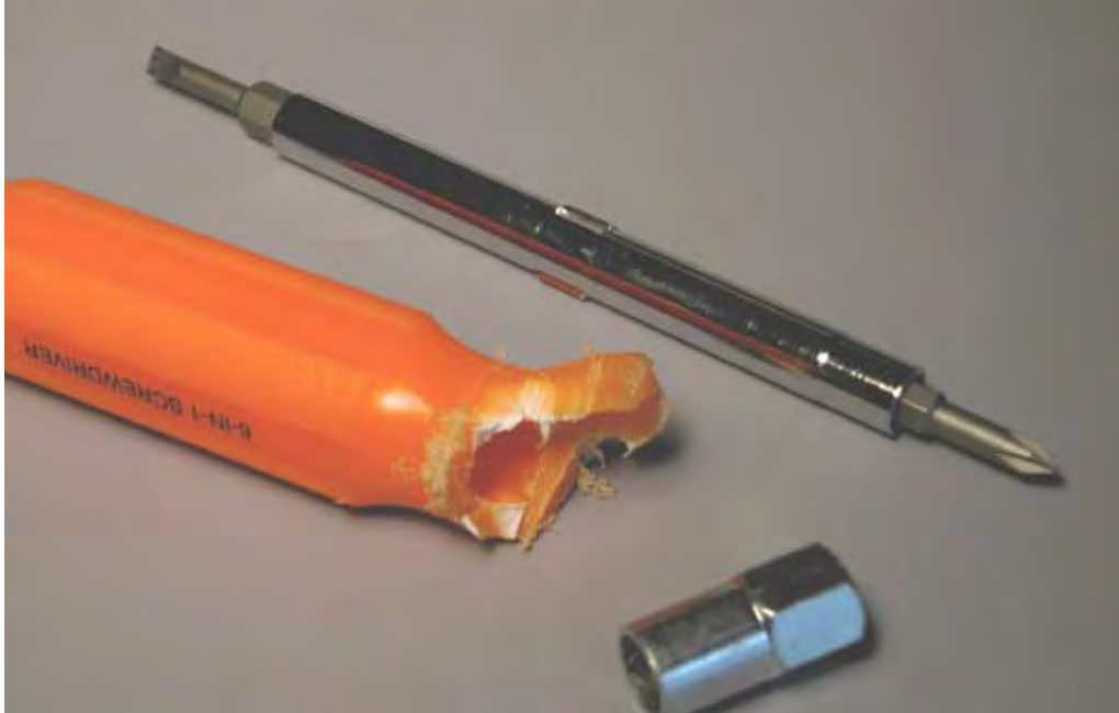
After sawing into the handle of a plastic screwdriver, salvage the nut (foreground), shaft, and drive points.
