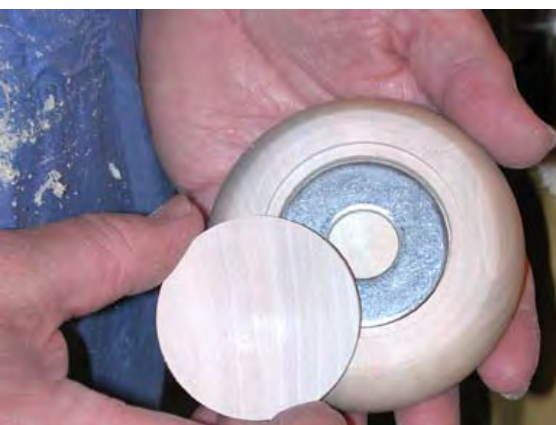
After adhering the washers, cover the base with the plywood cover.
