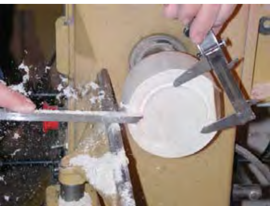
With a vernier scale, check the 2 1/8" diameter of the 1/8"-thick plywood cover.
