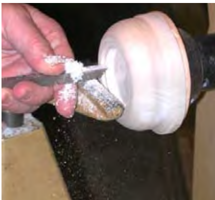
A square-end scraper provides an alternate way to cut a 2⅛" recess.
