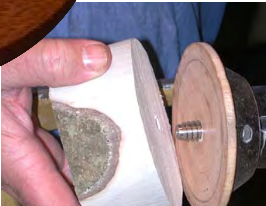
Attach your 2"-thick turning block to a screw chuck. With a ¼" plywood spacer on the screw chuck, the threads will grab about ½" of stock.
