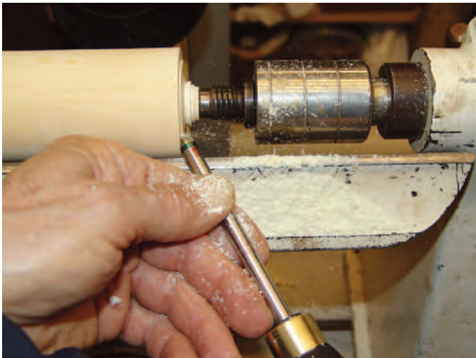
Facing cut: On an end-grain surface, align one triangular face with the surface. Drop the handle, then arch the cut toward the center.
