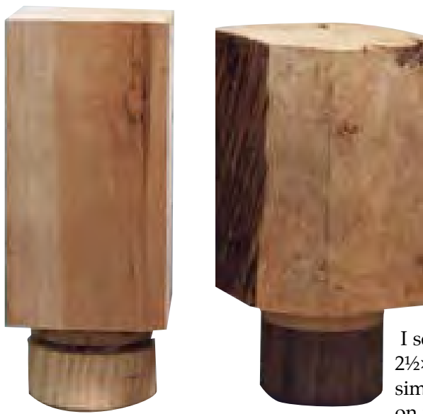
The cherry stem, left , and maple bowl, right , are shown mounted to waste blocks. Be sure to choose straight-grained stock.
