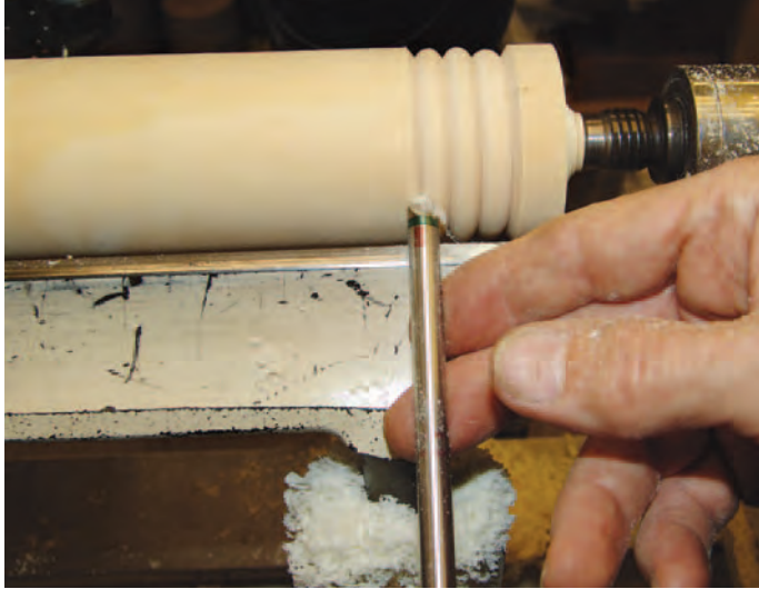
Bead step 1: After making a V-cut, swing the handle slightly toward the center of the bead.
