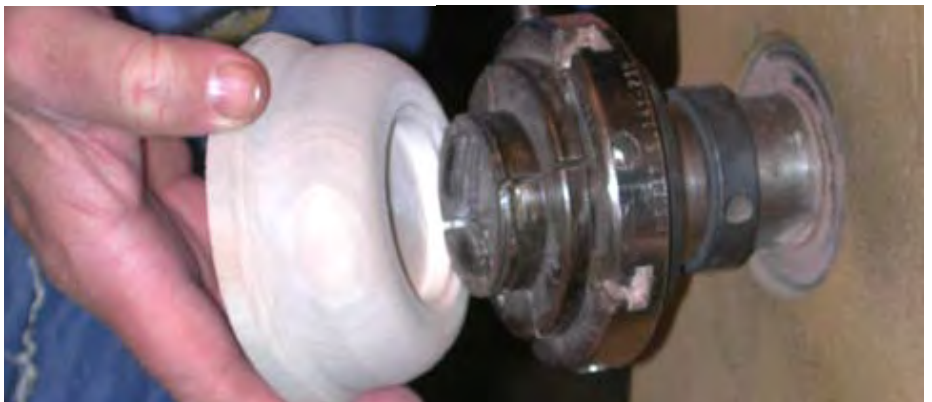
After shaping the bottom of the paperweight, mount the stock to an expanding chuck.
