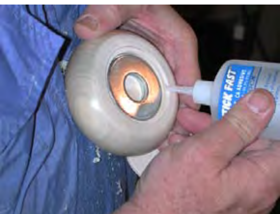
Use drops of cyanoacrylate (CA) glue to secure three washers in the recess.
