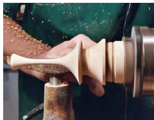
Use a spindle gouge to eliminate waste wood between the foot and your chuck. After doing this, you can undercut the foot to create a pleasing, stable base.
