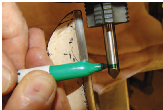
Use a Sharpie marker to guide your formation of three equal sides.
