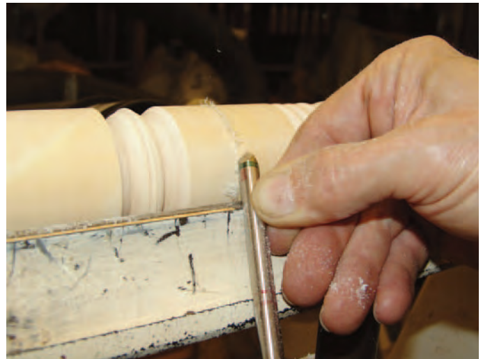
Planing cut: Place the triangular face of the tool flat on the surface. Advance the handle slightly in the direction of the cut.
