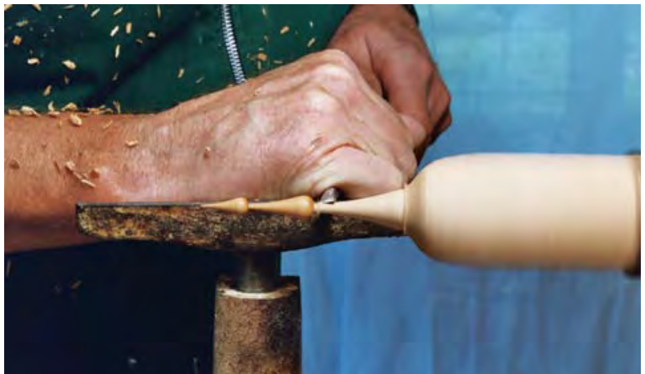
When turning the finial, always leave adequate mass at the base to dampen vibration. A small round skew and \frac{1}{2} " roughing-out gouge are ideal for this task.
