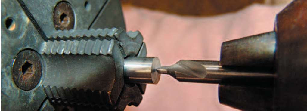
Mark the center of your high-speed steel with a carbide bit or diamond stylus.
