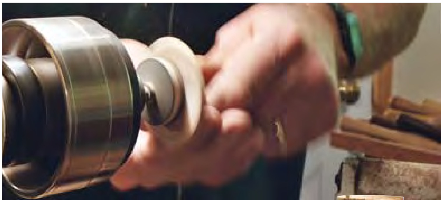
To sand the base of the foot, chuck a small sanding disc into your 4-jaw chuck.
