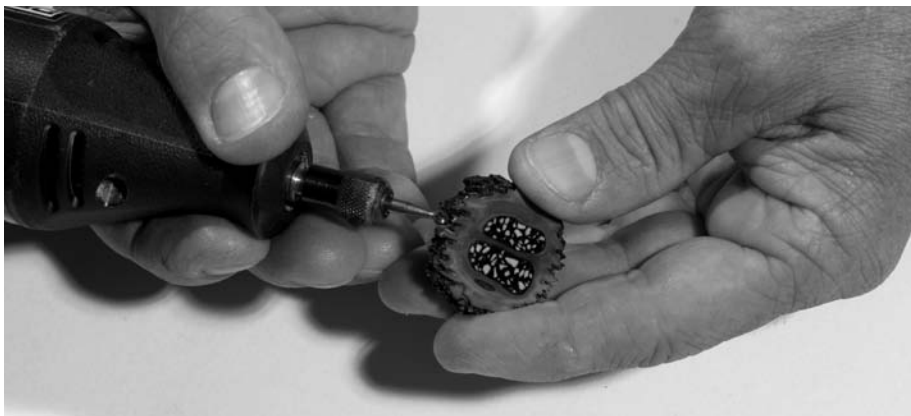
To prevent the drill bit from skating over the rough surface of the nut, the author first creates a dimple with a ball cutter chucked in a Dremel tool.
