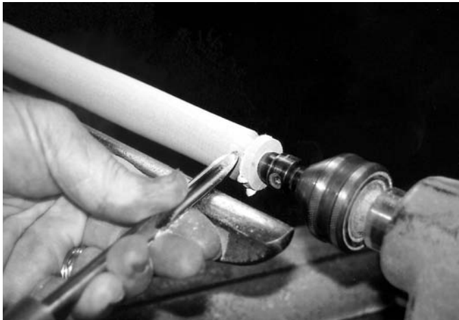
Begin shaping the icicle with the hat. The toolrest is mounted slightly below center, and the top of the icicle is secured by the tailstock.
