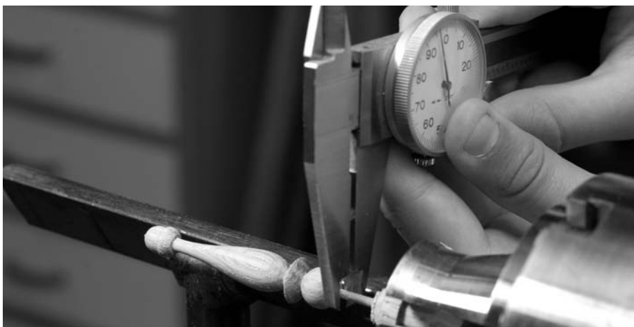
Lucas checks the accuracy of his cuts with a dial caliper set to .093-in.
