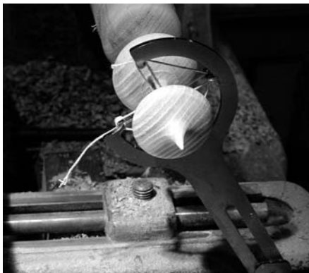
To secure the fragile trembleur, the author uses a traditional technique of using a string steady secured by a clove hitch, right, along the length of the spindle.
