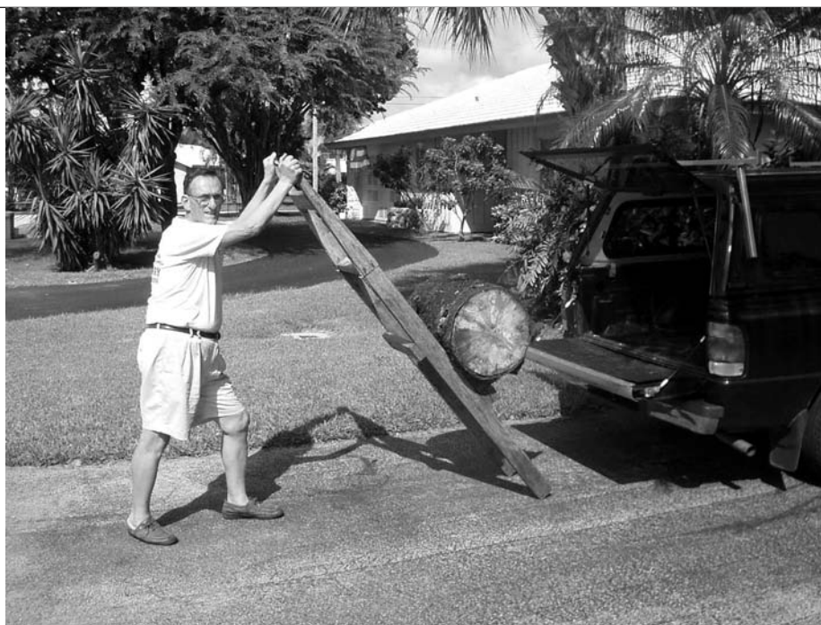
One-person log loader designed by Carl Schneider.
