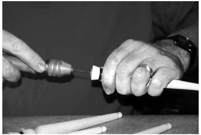
FINISHING THE ICICLE: The hat band is created before the blank is cut off the lathe by pressing a piece of masonite against the spinning wood, above, left. Be sure to predrill the hole for the slender eye hooks with a drill in a pin vise, above right, or a Dremel tool or other rotary tool.
