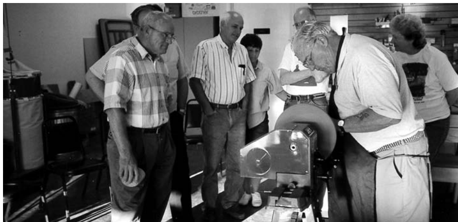
Marvin Murray demonstrating how to shape a foot with reverse turning. Photos: Ken Keoughan
