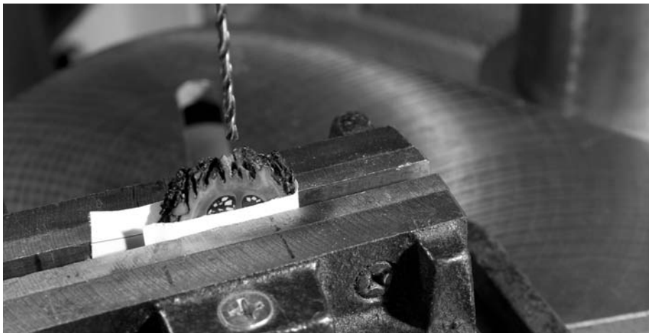
After protecting the flat faces with paper, the slice can be held in a vise and secured as the bit is guided into the recess created with the ball cutter.
