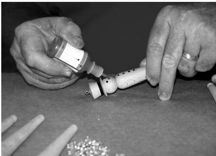
The button eyes and the nose, above left, are formed with a thick polymer puff paint; the mouth is done with a black Sharpie pen. The author finishes the ornaments by spraying on a couple of coats of Deft lacquer, above right.
