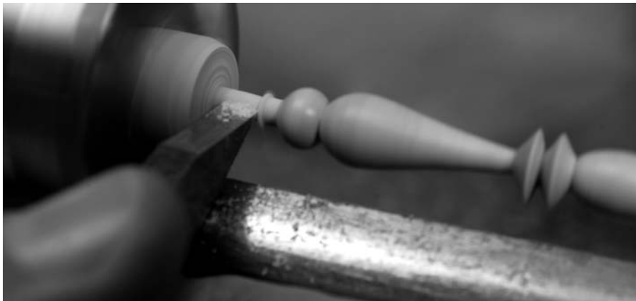
Cutting a tiny tenon: Lucas starts with a \frac{3}{16} -in. parting tool, which he rocks so it cuts on its corner.
