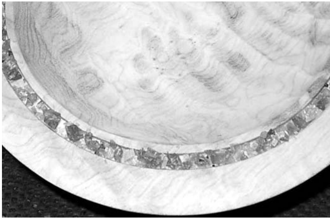
Largest pieces of crushed stone placed in slot prior to applying super-thin CA glue.
