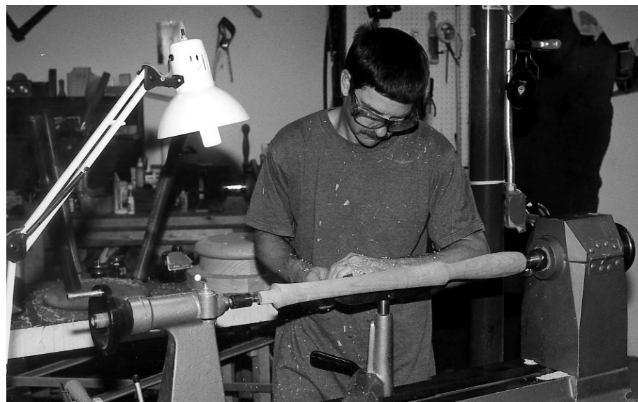
The two sides of stool making: Pleasant, graceful curves at the lathe, above, and a more violent approach to assembly, right. The trick is a tight fit without splits.
