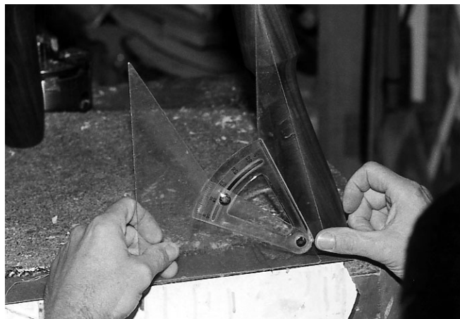
Find the angle between the leg and floor with an adjustable triangle. It will be slightly greater than the leg-to-seat angle.
