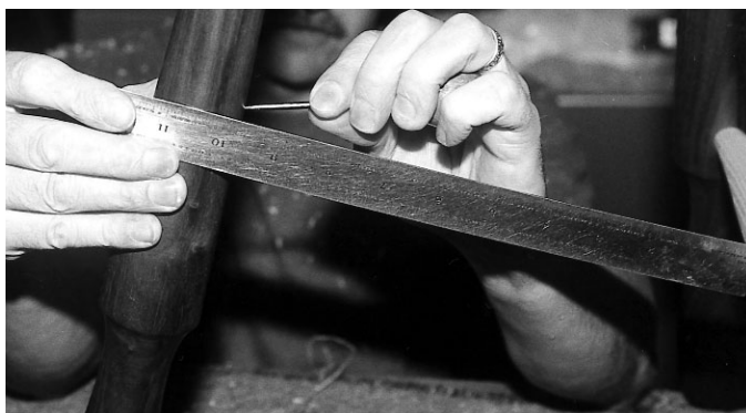
Locate the center rung with a straight edge run from the cross rung to the third leg and mark the location with an awl.
