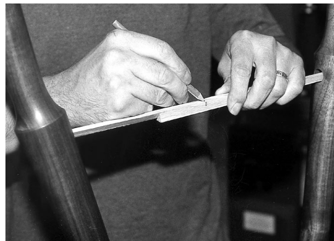
After boring holes in the legs for rungs, Scott determines the rung length with a simple story stick – two pieces of stock that slip into the holes and can be marked in the center, above.
