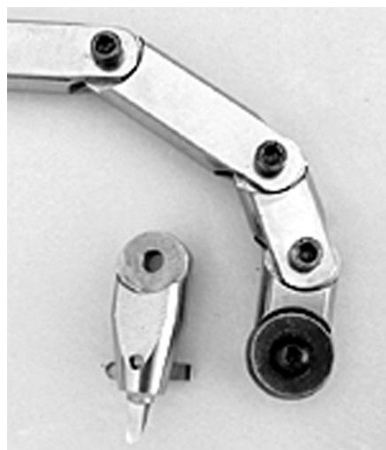
The circular scraper cuts less aggressively than the narrow cutter at right.
