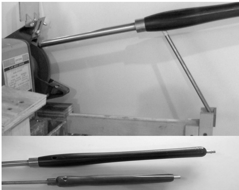
Self storing gouge sharpening jig.
