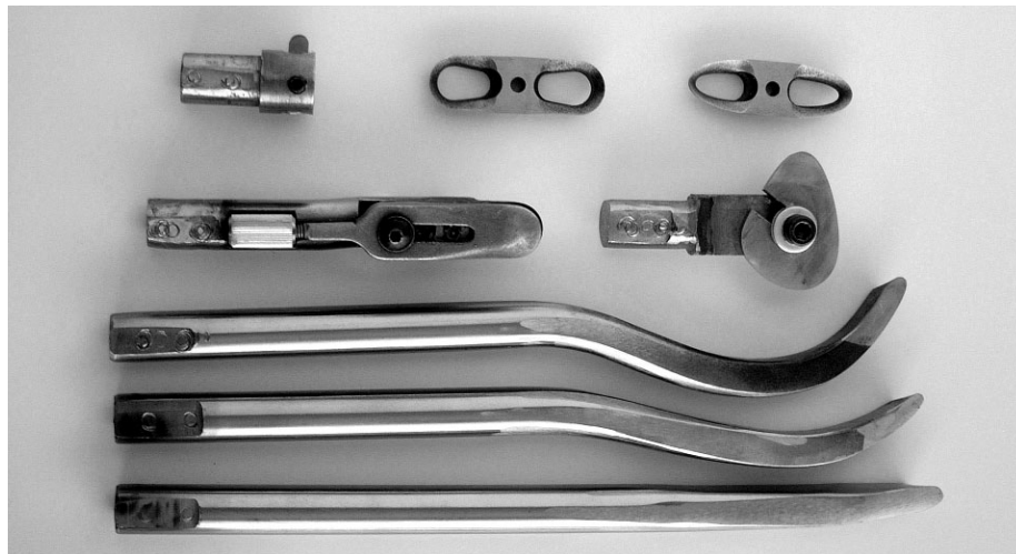
Boring bars and components: Top to bottom, left to right: Homemade holder with 3/16-in. metal working tool bit, round Exocet cutter, standard Exocet cutter; next line: Exocet assembly, homemade holder with teardrop scraper made from a planer blade; bottom section, set of 1/2-in. Kelton Hollowers.
