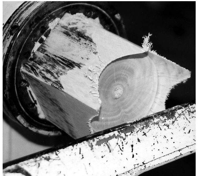
PHOTO 2: Inside almost finished. Note the tip of the peaks still have flat ends and uncut fibers on outside surface.
