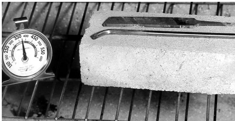
The metal can be tempered, a process which balances its edge-holding ability with toughness in a home-kitchen oven.
