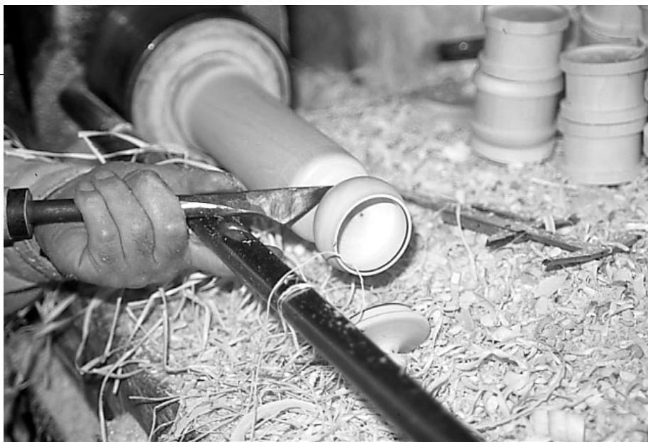
The outside of the box is finished and cut off with a large skew.
