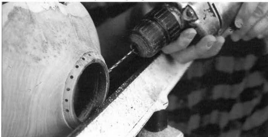
With the spindle locked and the drill positioned with a slight inward slant, the author begins drilling 1/8-in. diameter holes for the laces.
