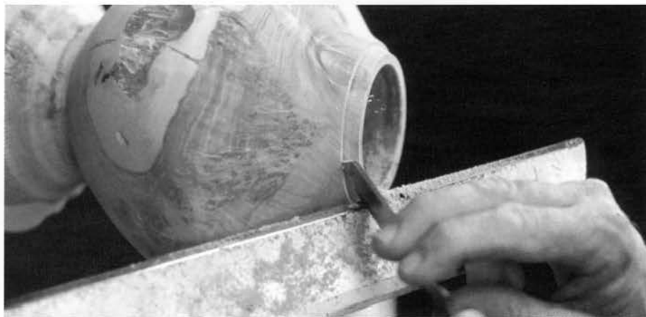
Use a 1/8-in. parting tool to cut the rabbet where the lacing holes will be drilled.
