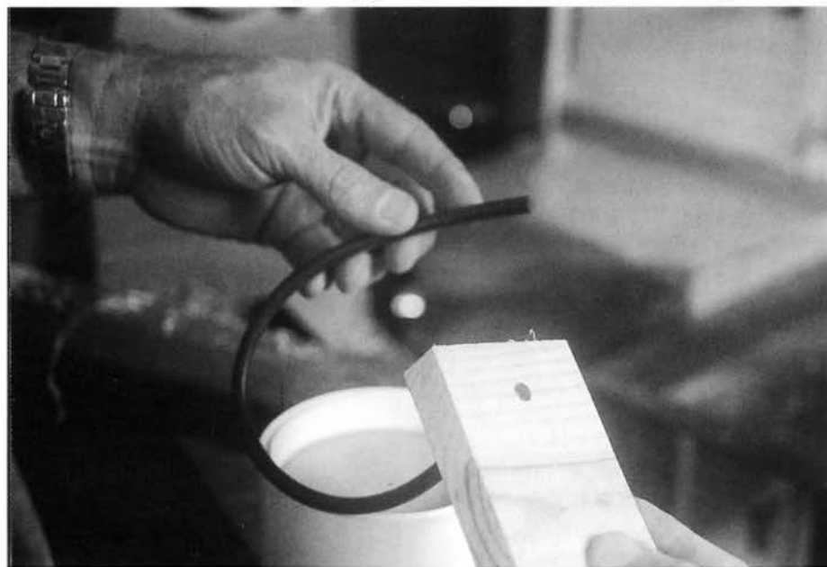
For a tight seal, both ends of the O-ring material must fit tightly together. To square the cut ends, the author fits the material through a hole drilled in a board, then uses that guide to square the material on a belt sander
