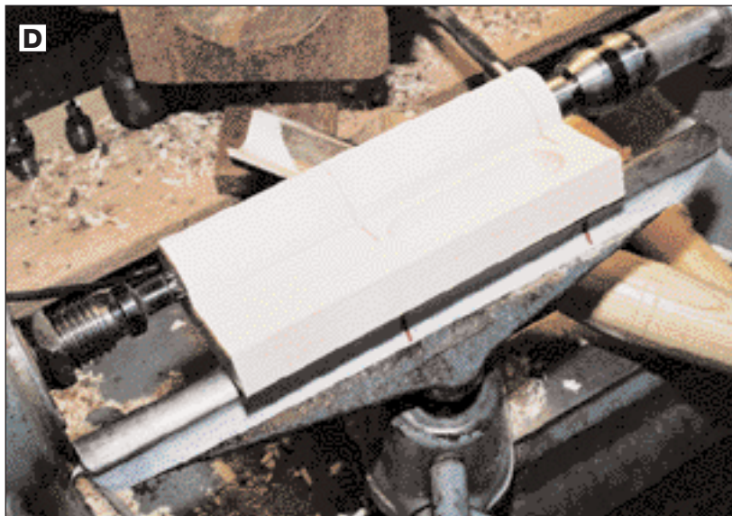
D With an extra blank, mark out the rattle ends on the blanks (pencil lines) and tool rest (red lines).
