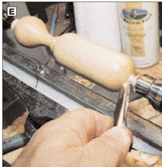
E With a 1/2" spindle gouge, part off the rattle end. A long fingernail grind guarantees success.
