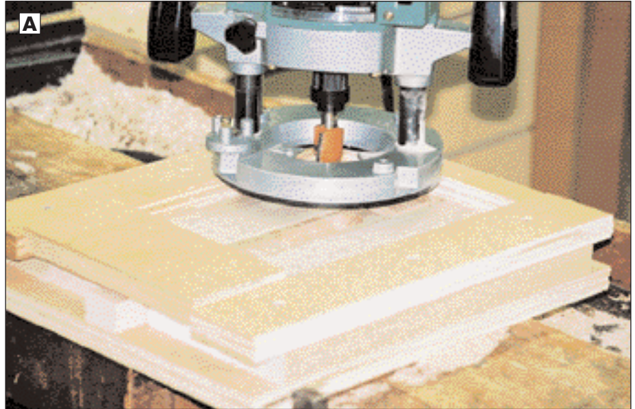
To rout the rattle cavity, use a 2\frac{1}{2} hp plunge router fitted with a 1" core-box bit.
